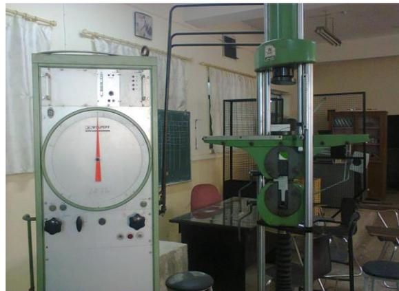
Figure(2):WOLPERT tensile testing machine
