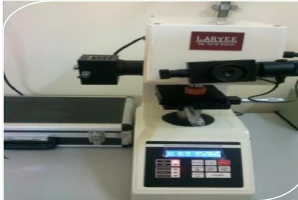
**Figure (6) : Digital Micro Vickers hardness tester “LARYEE“.**
