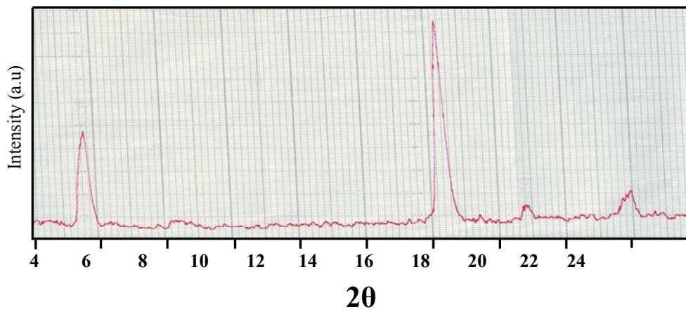
**Figure( 5 ):XRD for PCVT thin film at R.T**
