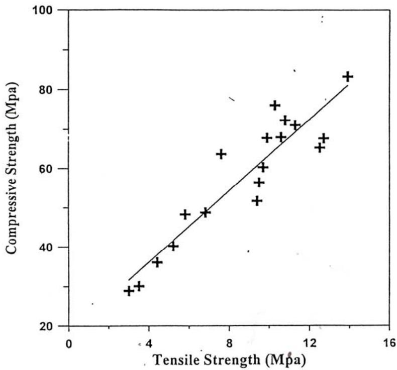
Figure (5) Shows a mathematical model for the relationship between tensile strength and compressive strength for different mixes of PMC.
