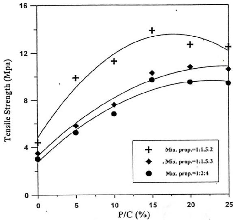
Figure (4) The effect of the increase in (P/C) on tensile strength of (PMC)
