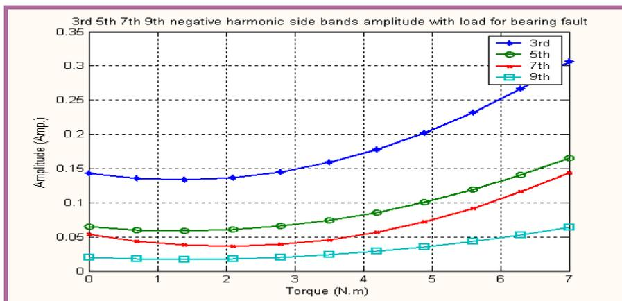
**Figure (15) Changing the Amplitude of the negative harmonic with load for bearing fault with 3<sup>rd</sup> 5<sup>th</sup> 7<sup>th</sup> 9<sup>th</sup> harmonic**
