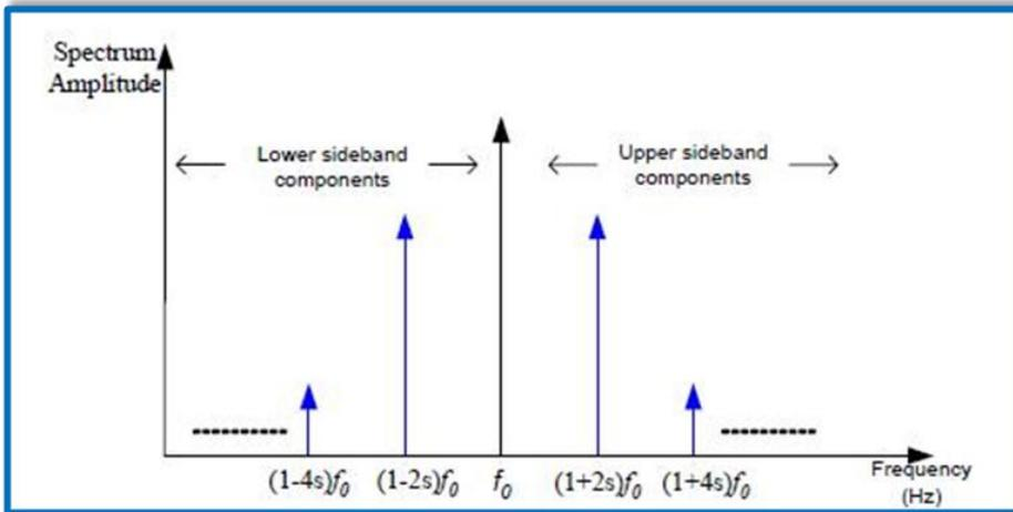
**Figure (9) sideband components around the fundamental frequency**
