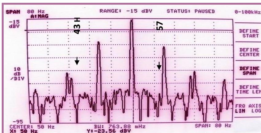
**Figure (16) Bearing fault at no load, center=50, span=80**
