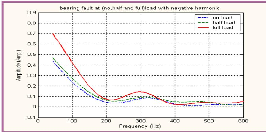
**Figure (14) Changing the Amplitude of the positive harmonic with load for bearing fault with 3<sup>rd</sup> 5<sup>th</sup> 7<sup>th</sup> 9<sup>th</sup> harmonic**
