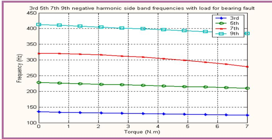
Figure (11) Changing the Frequencies of the negative harmonic with load for bearing fault with 3<sup>rd</sup> 5<sup>th</sup> 7<sup>th</sup> 9<sup>th</sup> harmonic
