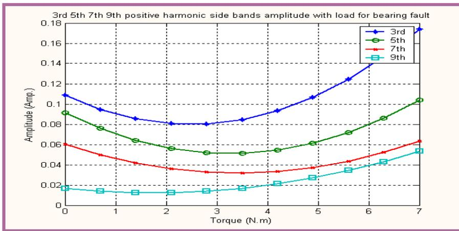
Figure (12) Changing the amplitudes with Frequency of the positive harmonic with (no, half and full) load for bearing fault
