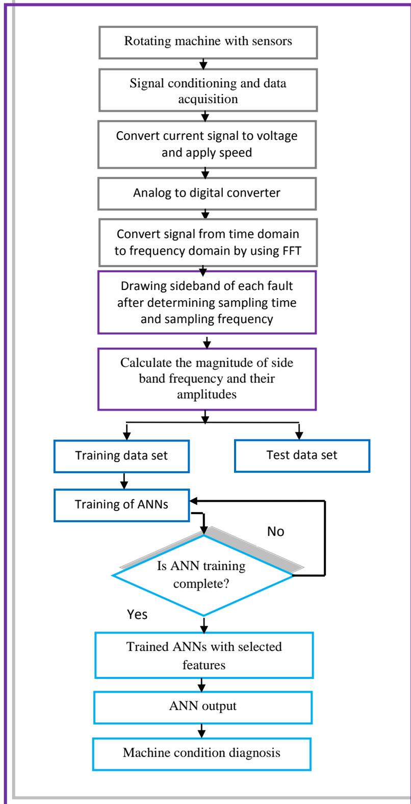
Figure (18) Algorithm of monitoring and diagnostic process
