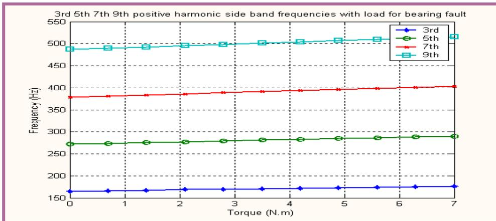
**Figure (10) Changing the Frequencies of the positive harmonic with load for bearing fault with 3<sup>rd</sup> 5<sup>th</sup> 7<sup>th</sup> 9<sup>th</sup> harmonic**
