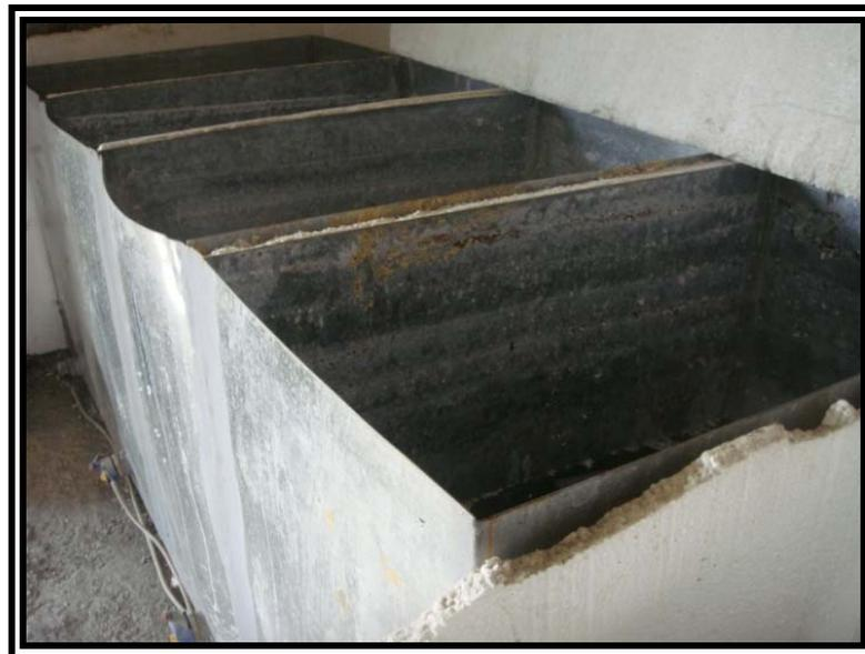
Figure (2): Water Curing Tank Divided to Various Temperatures
