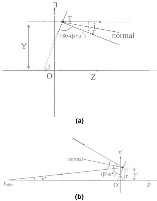
**Fig. (3) Ray reflection at the Cassegrainian reflectors (a) Reflection at the Cassegrainian primary reflector (b) Reflection at the Cassegrainian secondary reflector**
