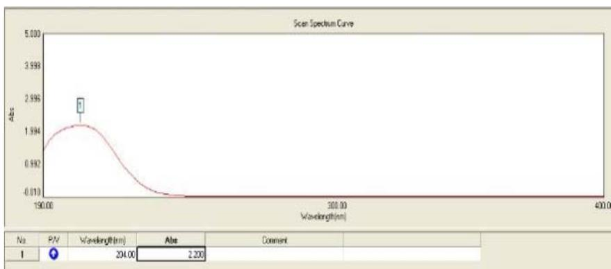
Figure (4b) The absorption spectrum of the BaNO<sub>3</sub> at concentration of 25 ppm
