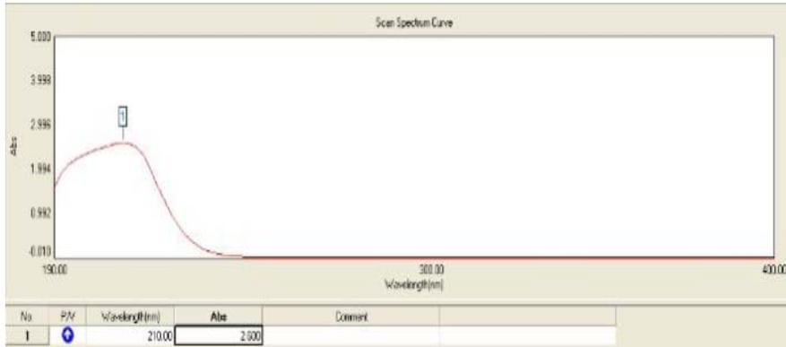
Figure (4c) The absorption spectrum of the BaNO<sub>3</sub> at concentration of 50 ppm
