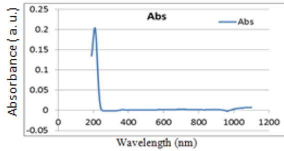
Figure (3b) The absorption spectrum of the NaNO<sub>2</sub> at concentration 20 ppm
