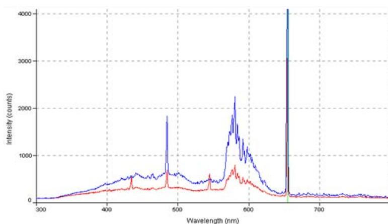
**Figure(5) Differential absorption cross-sections of different gas species (NO<sub>x</sub>) at 4m in the laboratory.**
