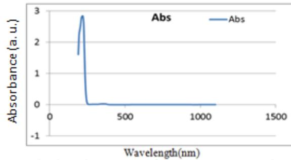
Figure (3f) The absorption spectrum of the NaNO<sub>2</sub> at concentration 150 ppm
