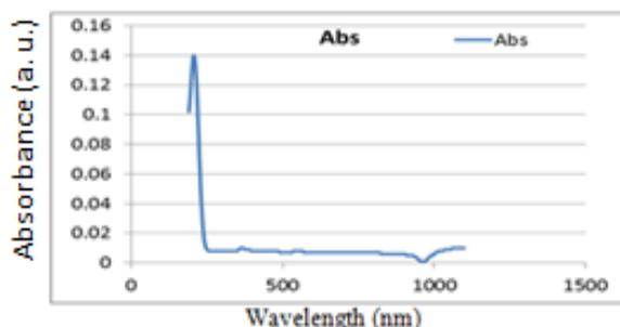
Figure (3a) The absorption spectrum of the NaNO<sub>2</sub> at concentration 15 ppm
