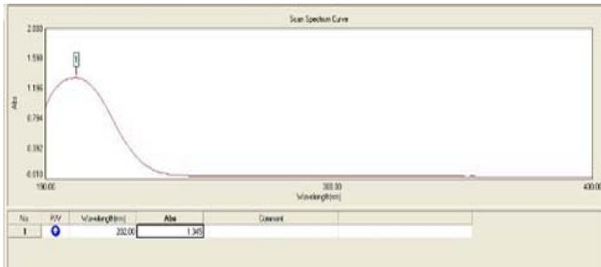
Figure (4a) The absorption spectrum of the BaNO<sub>3</sub> at concentration of 15 ppm
