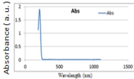
Figure (3d) The absorption spectrum of the NaNO<sub>2</sub> at concentration 100 ppm
