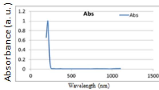
Figure (3c) The absorption spectrum of the NaNO<sub>2</sub> at concentration 55 ppm
