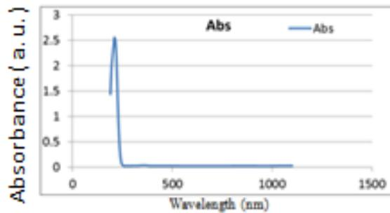
Figure (3e) The absorption spectrum of the NaNO<sub>2</sub> at concentration 125 ppm
