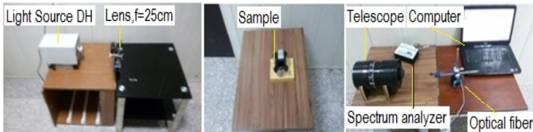
Figure (2): Overall devices of the DOAS system model
