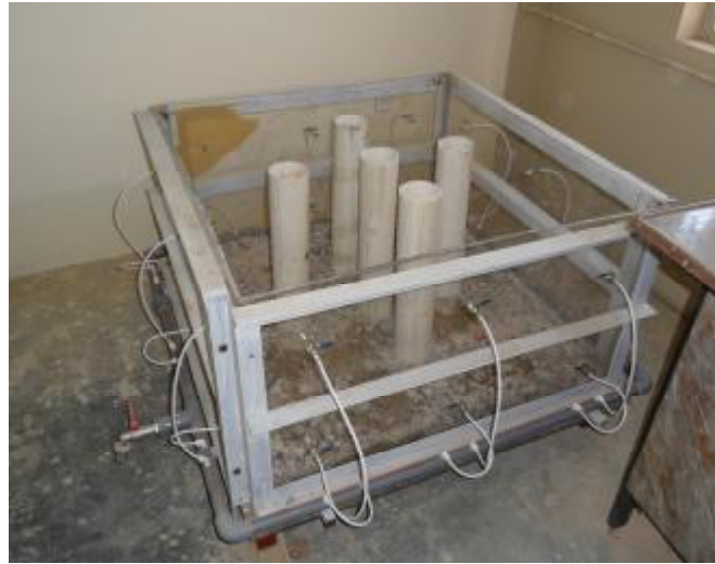
Figure (5) Photos represent the frame steel of model and water discharge valves.
