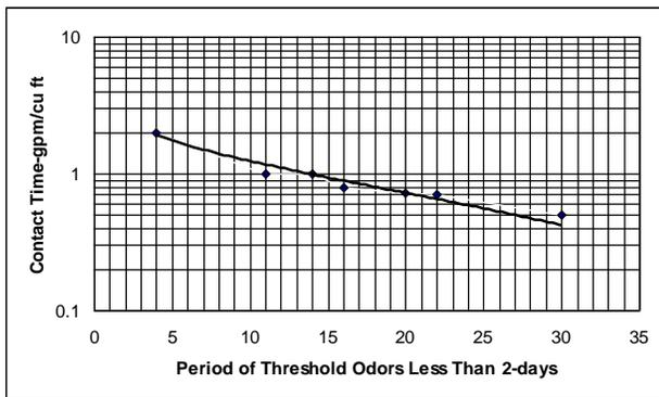
Fig.3: Relationship of Contact Time to Reduction of Threshold Odor at (Nitro, W. Va) (Dostal et al, 1965).
