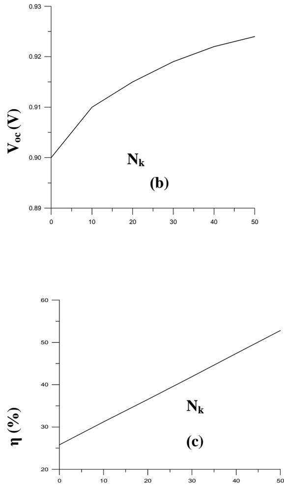
**Figure 5: short-circuit current (a), open-circuit voltage (b) and efficiency (c) as function of number wells.**
