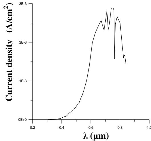
**Figure 3: total current density for a 50 QWs as function of wavelength.**
