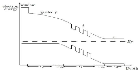
Figure 1: QWSC band diagram.
