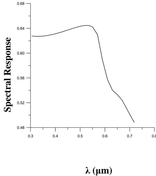
**Figure 4: total spectral response for a 50 QWs as function of wavelength.**
