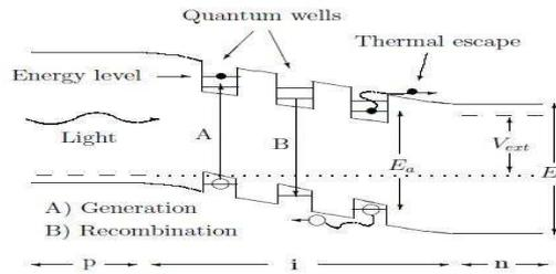
**Figure 2: schematic of the QWSC structure, absorption, recombination and escape mechanisms.**
