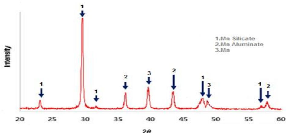
**Figure 1 .** XRD pattern of steel slag.
