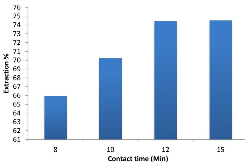
**Figure 9.** Effect of the contact time on the extraction of Mn.
