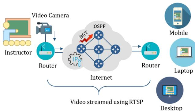
Figure 3: Conceptual network diagram
