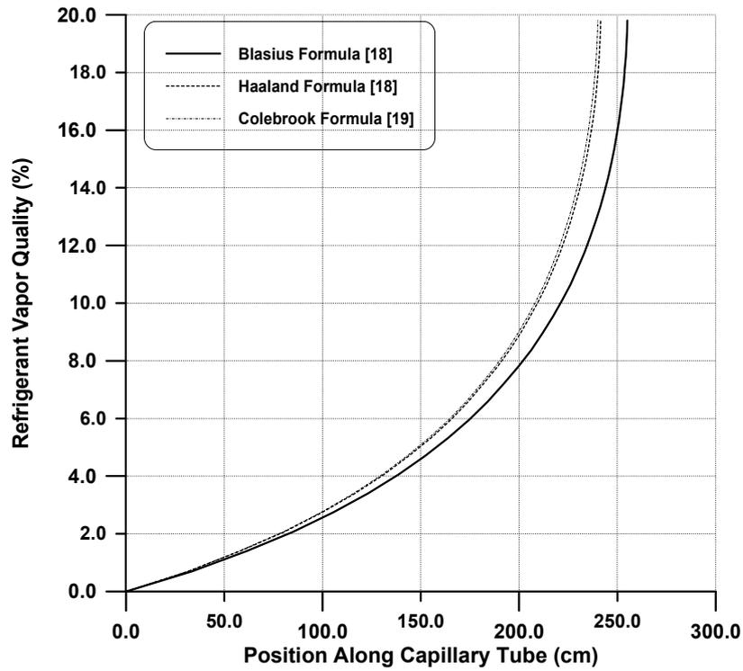
Figure (7): The present model predicted refrigerant (R-22) vapor quality distribution for Sami et al. [21] operating conditions.
