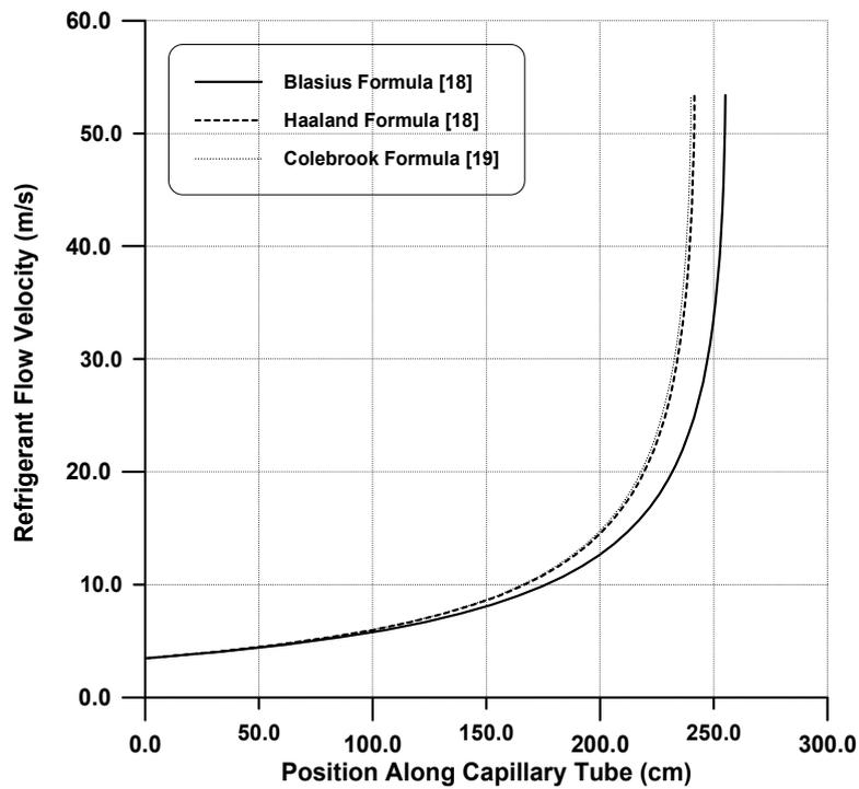
Figure (6): The present model predicted refrigerant (R-22) velocity profile for Sami et al. [21] operating conditions of the capillary tube.
