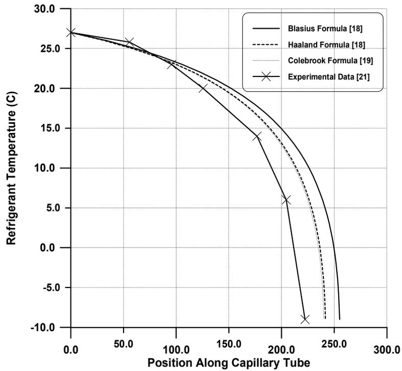
Figure (5): Comparison of the predicted temperature profile for the refrigerant R-22 with that of Sami et al. [21] experimental data.
