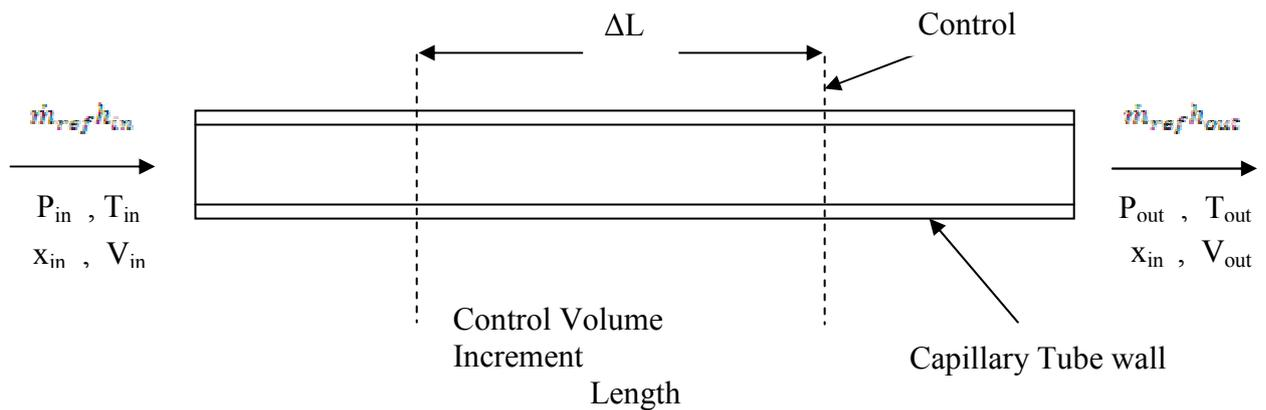
Figure (1): A Schematic diagram for the control volume of fluid flowing inside the capillary tube.
