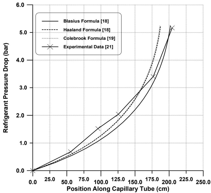
Figure (9): Comparison of predicted pressure drop for refrigerant (R-407C) of the present model with Sami et al. [21] experimental
