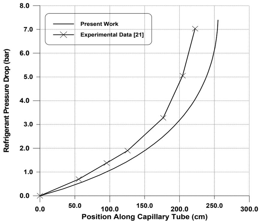
Figure (4): Comparison of the predicted refrigerant (R-22) pressure drop profile with the experimental data of Sami et al. [21].
