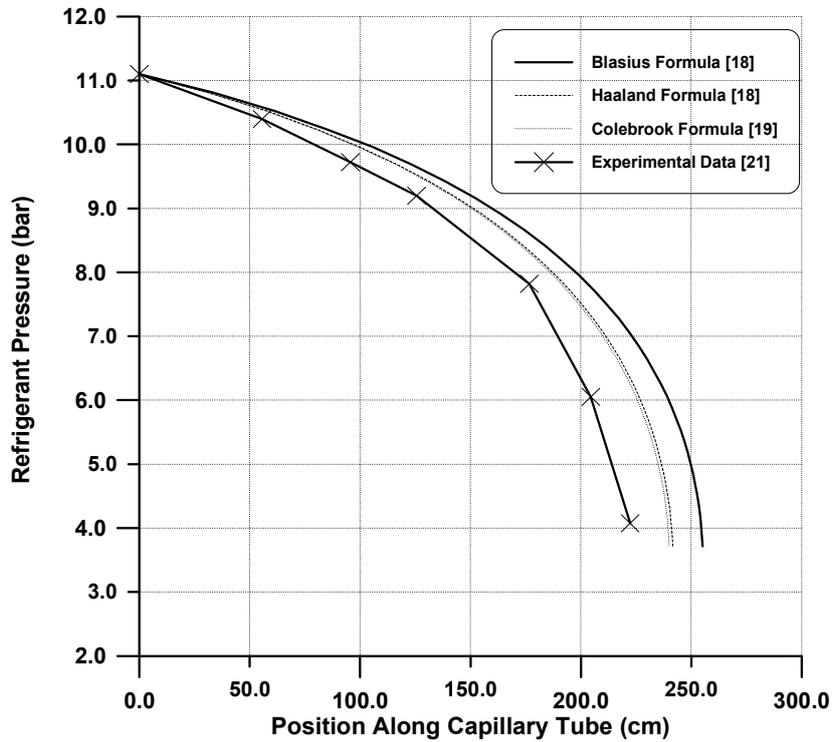
Figure (3): The predicted pressure profile of the refrigerant (R-22) compared to the data of Sami et al. [21] for different friction factor estimation methods.
