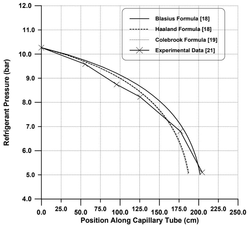
Figure (8): Comparison of predicted pressure profile for refrigerant (R-407C) of the present model with Sami et al. [21].
