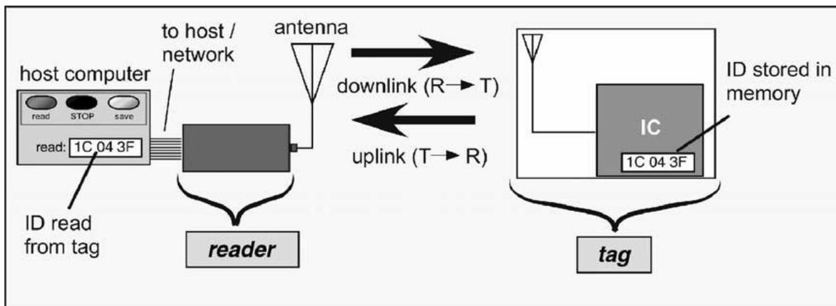
Figure 1. Basic Operations of RFID [3]
