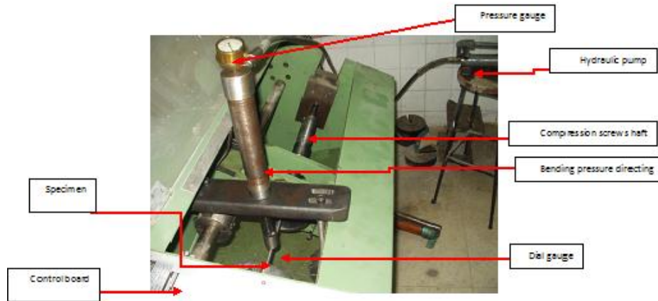
Figure (1) the dynamic buckling test rig.
