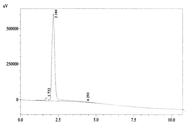
**Fig. (4) HPLC Chromatogram for acenaphthene at 228nm.**
