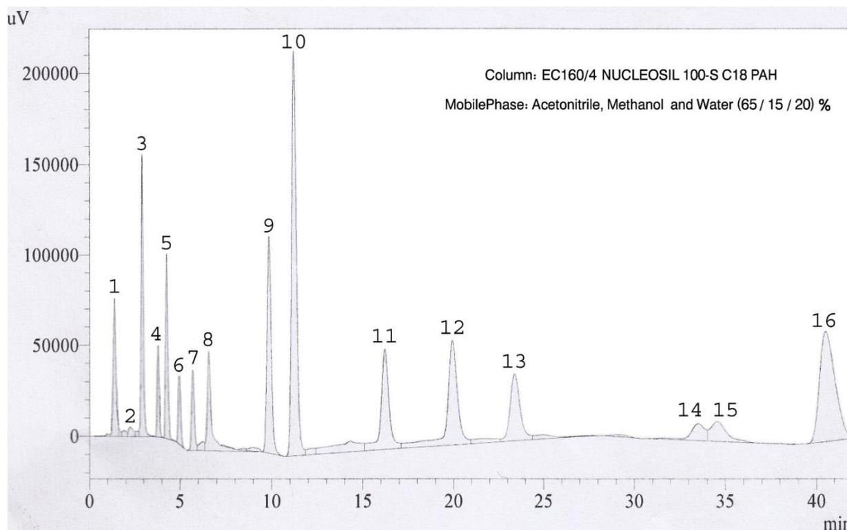
**Fig. (2) HPLC Chromatogram for 16 PAHs(5mg/l) at 260nm, flow rate 1 ml/min, mobile phase (Acetonitrile 65%, Methanol 15% and Water 20%)** 1-Naph. 2- Ace. 3- Acy.4- Fln. 5-Phe. 6- Anth.7- Flan. 8- Py. 9- Ch. 10- B[a]anth. 11- B[b]flan. 12- B[k]flan. 13- B[a]p 14- B[ghi]pyr. 15- D[a,h]an. 16- I[123-cd]py.
