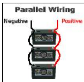
Fig .9: The parallel wiring
