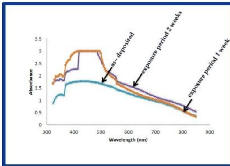
**Figure (3) typical optical absorption spectra for CdTe thin films, Corresponding to different values of the exposure period of reference Films with  $\gamma$ -irradiation after one week.**
