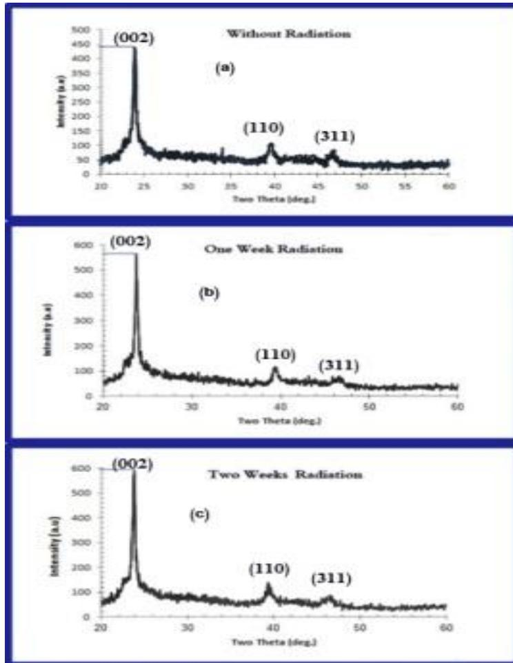
Figure (3) XRD patterns of a: deposited reference films without  $\alpha$ -irradiation b: deposit reference films without  $\alpha$ -irradiation after one week c: reference films without  $\alpha$ -irradiation after two week.
