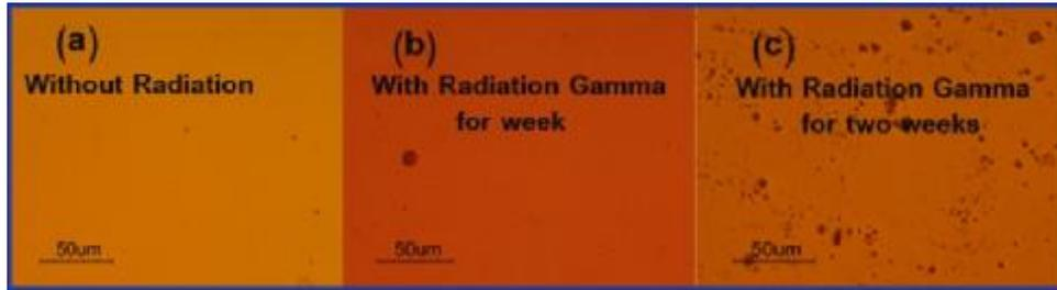
Figure (1) : Image of CdTe thin films without  $\gamma$ -irradiation, b: Image of CdTe thin films with  $\gamma$ -irradiation for week and c: Image of CdTe thin films with  $\gamma$ -irradiation for two week.
