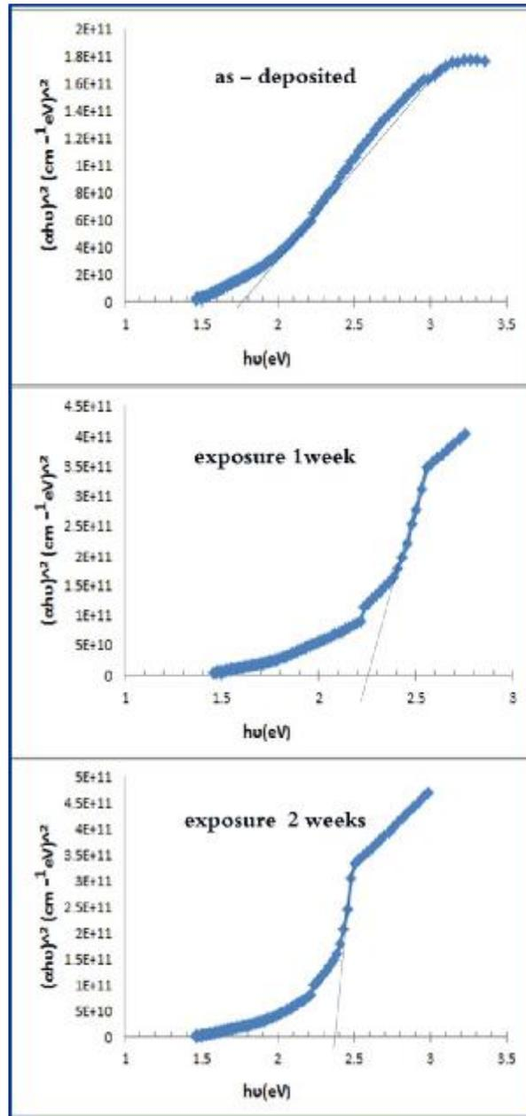
Figure (4) Plots of  $(ah\nu)^2$  vs  $h\nu$  for CdTe thin films, corresponding to different values of the exposure oeriod of gamma radiation dose.
