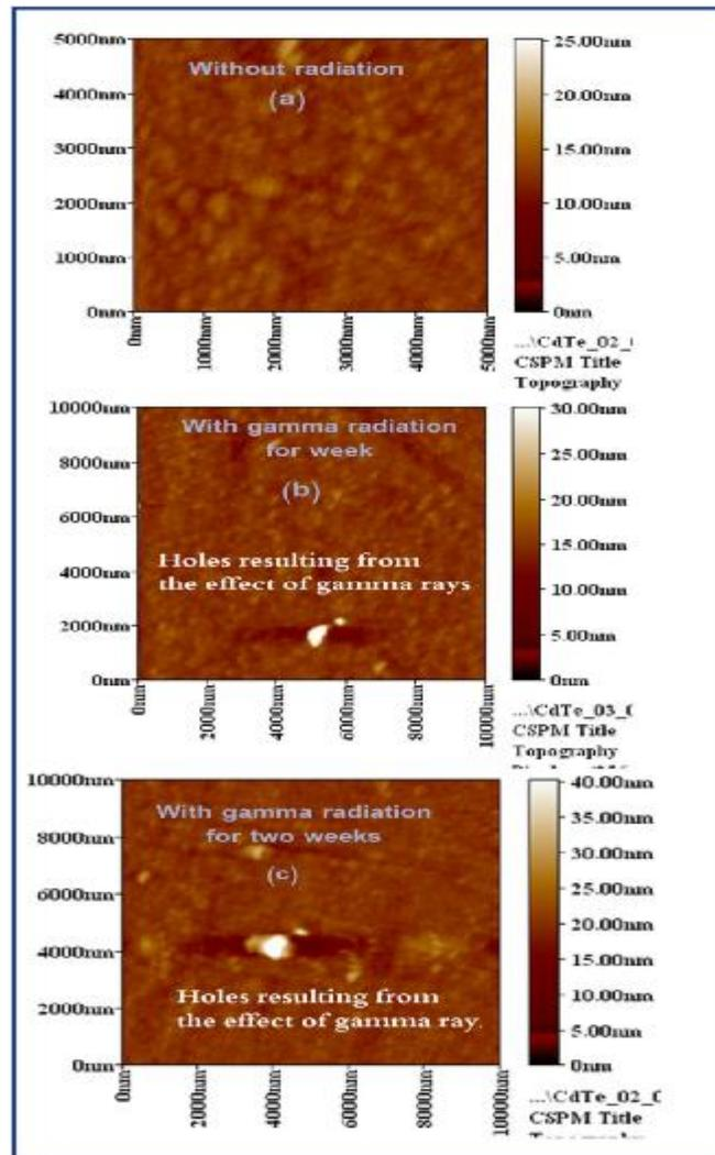
Figure (2) Atomic force microscope (AFM) Image of CdTe thin film
