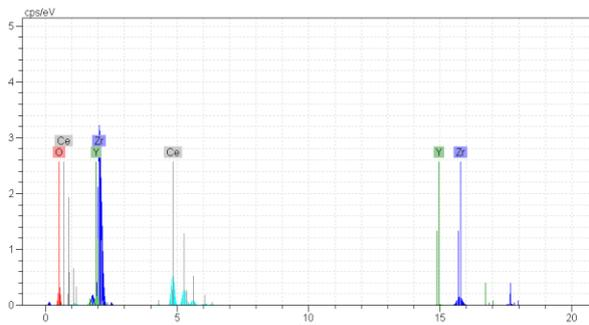
**Figure 10: Typical EDS analysis of plasma sprayed coating showing the elements.**
