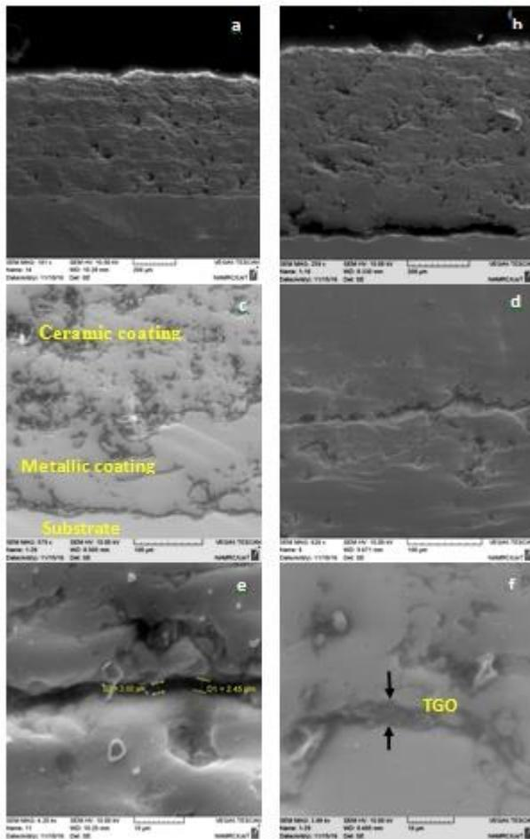
**Figure 4: Typical SEM photographs of transverse sections of plasma sprayed (CYSZ); (a) and (b), (c) and (d) higher magnification of interfaces between coatings, (e) and (f) thermally grown oxide layers.**
