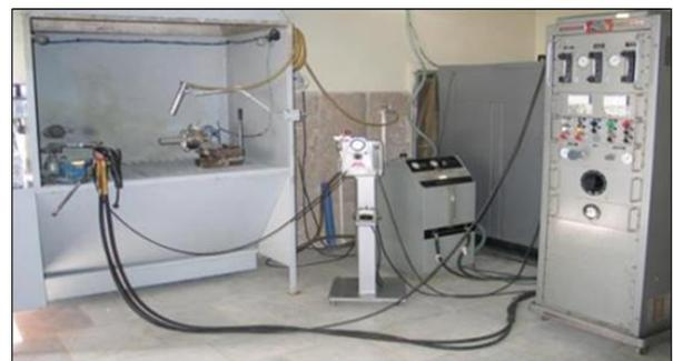
**Figure 1: Plasma sprayed unit used in this investigation.**
