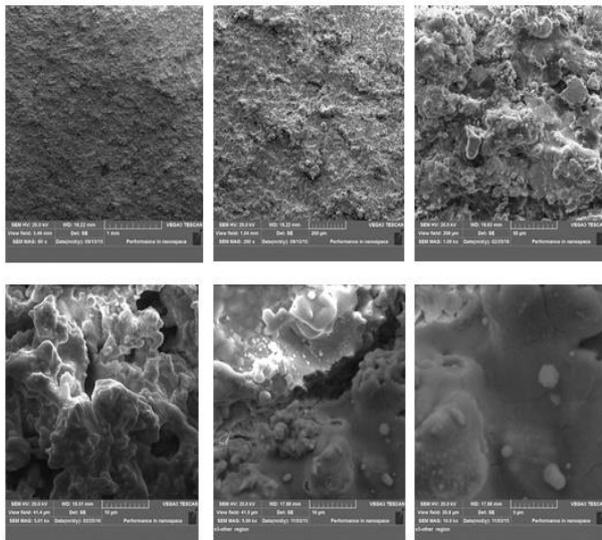
**Figure 2: Typical SEM photographs of upper surface plan views of plasma sprayed zirconia-20 wt% ceria- 3.6 wt% yttria (CYSZ) at different magnifications showing the heterogeneous distribution of melted splats, semimelted and unmelted particles.**
