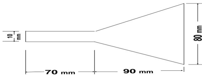
**Fig. 5 E-plane flared side of pyramidal horn antenna**
