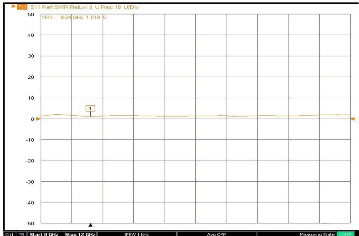
Fig. 8 Voltage Standing Wave Ratio (VSWR) result
