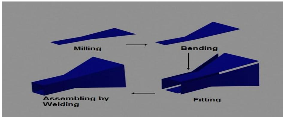
**Fig. 6 Technological path for horn antenna fabrication**
