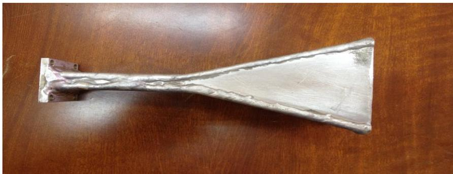
**Fig. 7 Assembled pyramidal horn antenna**
