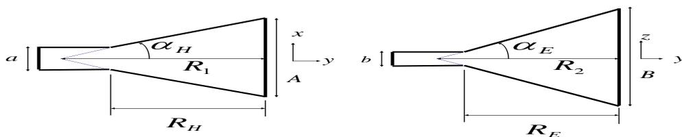
**Fig. 3 Geometry of a pyramidal horn**
