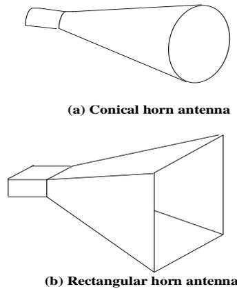
**Fig 1 Main types of horn antenna**
