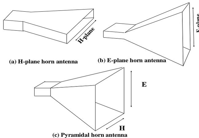
**Fig. 2. Types of rectangular horn antenna**
