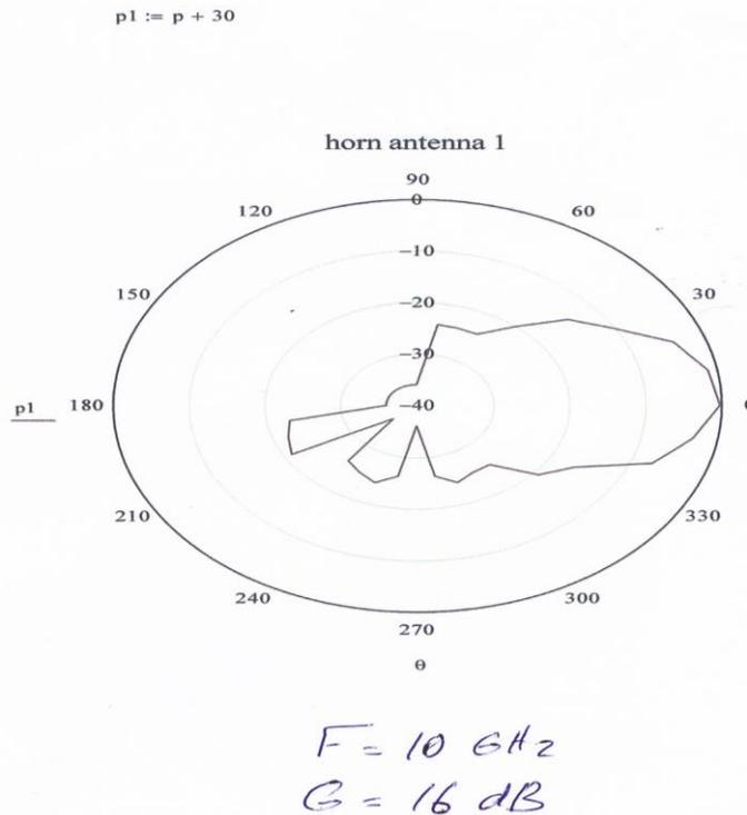
**Fig. 11 Radiation pattern of the pyramidal horn antenna, indicating the values of gain, side lobes level, and Half power beam width.**
