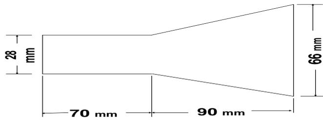
**Fig. 4 H-plane flared side of pyramidal horn antenna**
