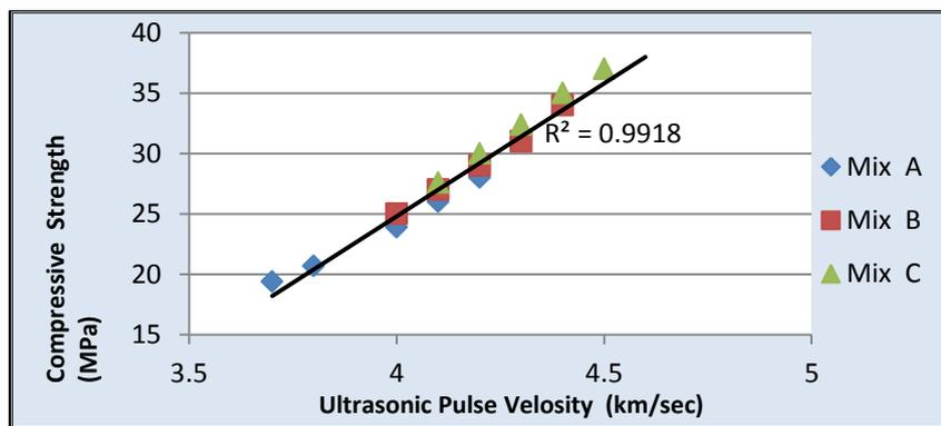
Figure (7) Relationship of UPV and the compressive strength
