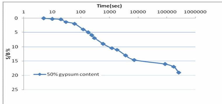
**Fig (5):** Collapse for soil with 50% gypsum content using the new device for collapse test.(soaking stress=100kPa, soil density=17.3kN/m<sup>3</sup>).
