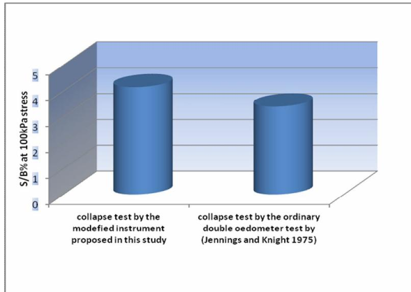
**Fig (11):** Collapse measuring using the MCT device proposed in this study, compared with that measured using the ordinary double oedometer collapse test, proposed by Jennings, J.E. and Knight, K. 1975) in measuring collapsibility of gypseous soil.(G.C=30%, soaking stress=100kPa).
