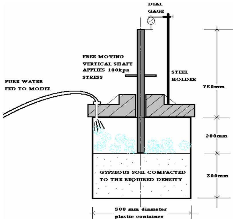
**Fig. (2-b):** parts and mechanism of (MCT) proposed in this study.
