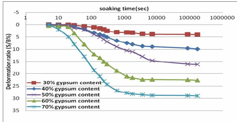
**Fig (8):** Results of laboratory test on model samples to simulate the collapsibility of gypseous soil with different gypsum content using MCT device.(stress level=100kPa, soil density=17.3kN/m<sup>3</sup>).
