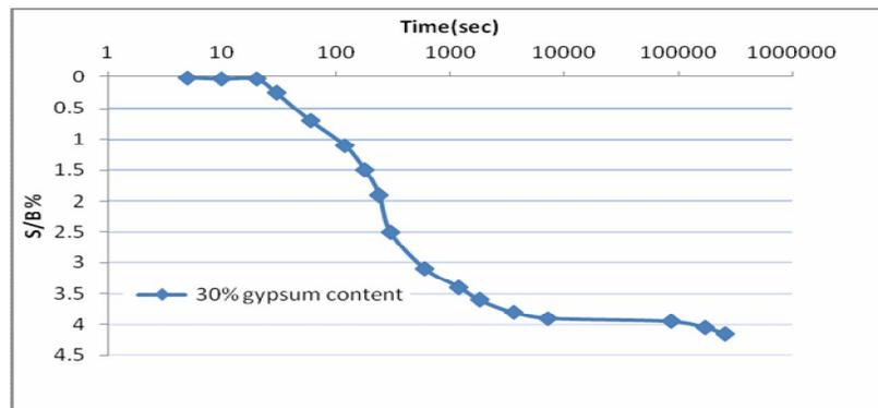
Fig (3): Collapse for soil with 30% gypsum content using the new device for collapse test.(soaking stress=100kPa, soil density=17.3kN/m<sup>3</sup>).
