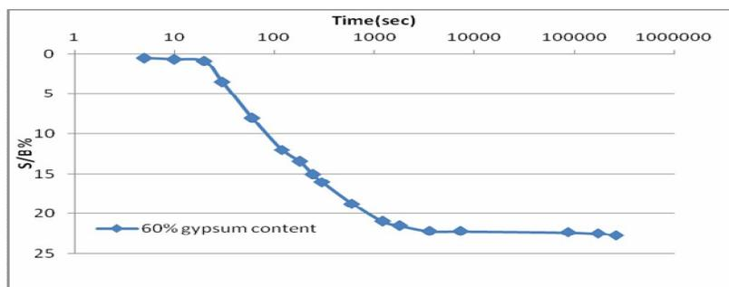
**Fig (6):** Collapse for soil model with 60% gypsum content using the new device for collapse test.(soaking stress=100kPa, soil density=17.3kN/m<sup>3</sup>).
