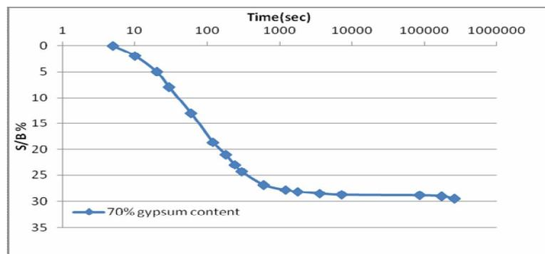
**Fig (7):** Collapse for soil model with 70% gypsum content using the new device for collapse test.(soaking stress=100kPa, soil density=17.3kN/m<sup>3</sup>).
