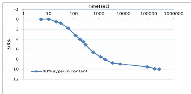
Fig (4): Collapse for soil with 40% gypsum content using the new device for collapse test.(soaking stress=100kPa, soil density=17.3kN/m<sup>3</sup>).
