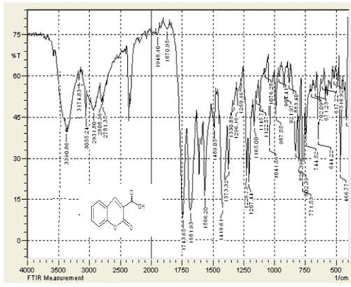
Fig.(1) FT- IR Spectrum for Compound (K)
