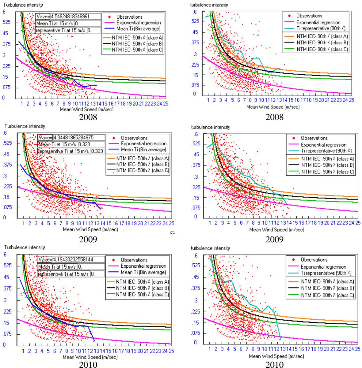
Figure 5- Turbulence intensity as a function of mean w. speed belongs to Nasiriyah site for large wind turbine.
