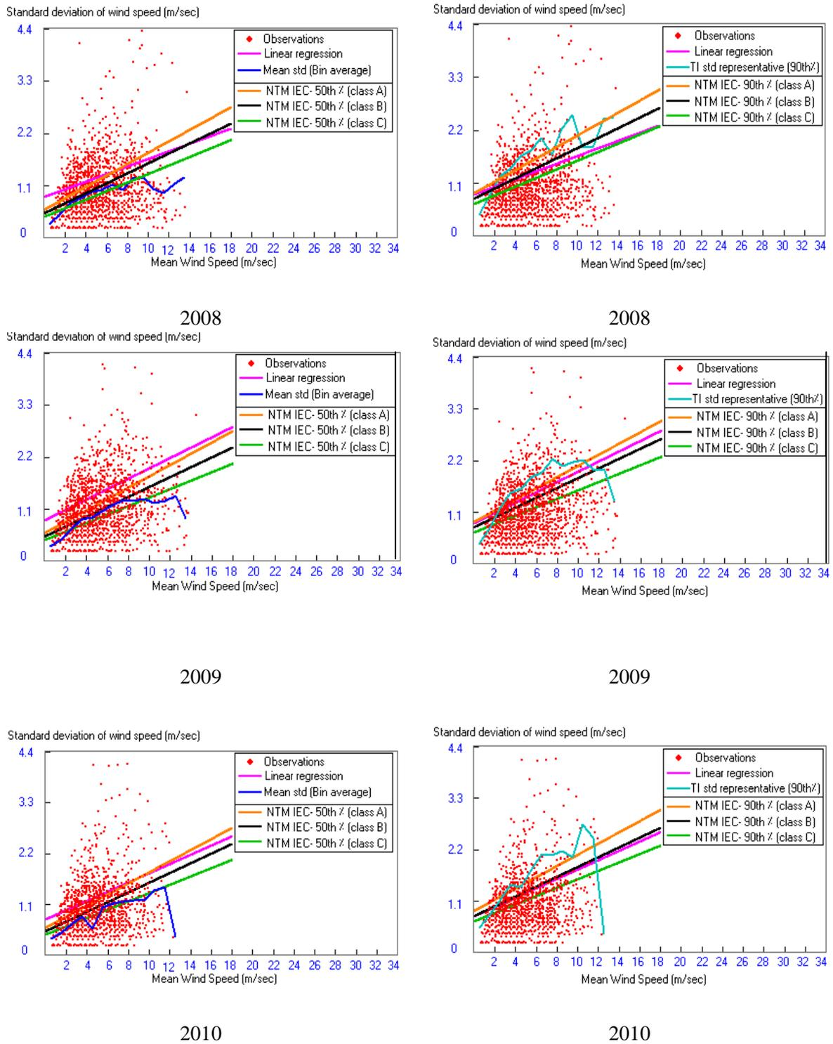
**Figure 3-** Standard deviation of w. speed as a function of mean w. speed belongs to Nasiriyah site for large wind turbine.
