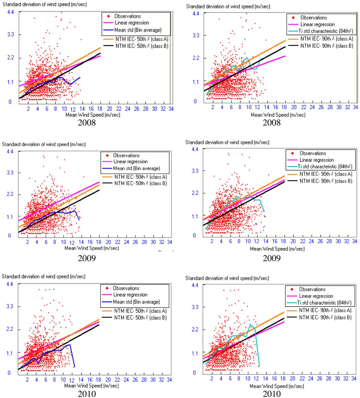
**Figure 4-** Standard deviation of w. speed as a function of mean w. speed belongs to Nasiriyah site for small wind turbine
