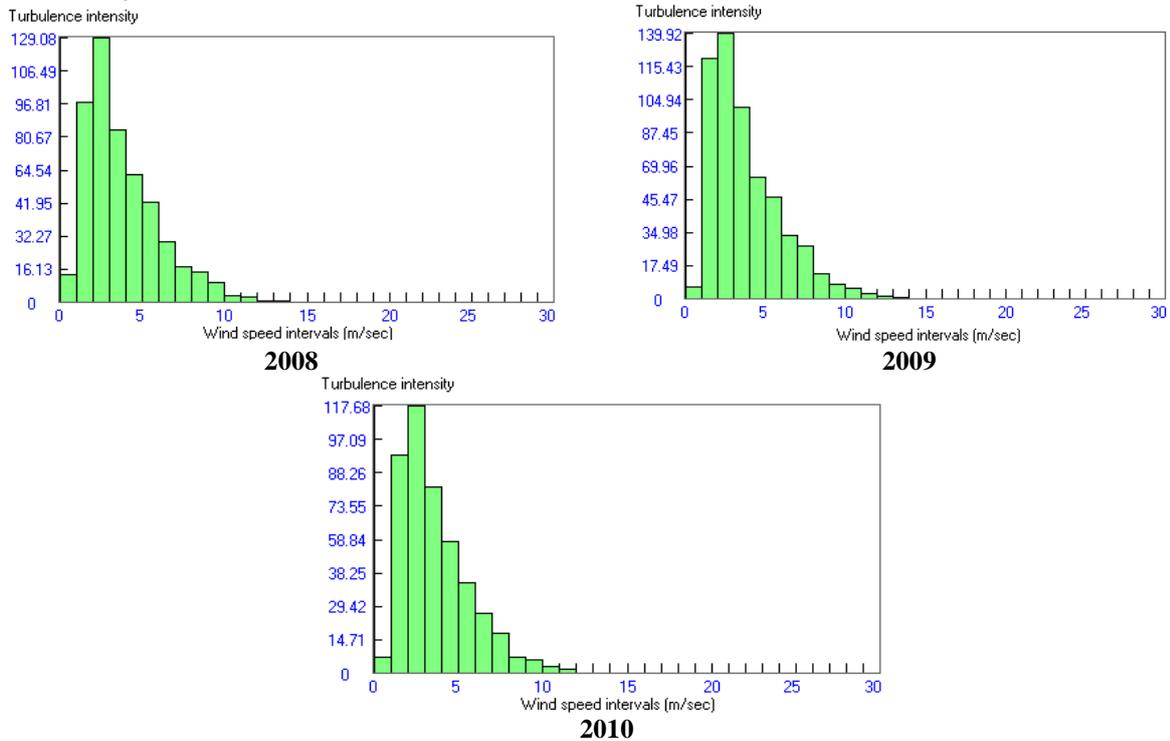
**Figure 8-** Turbulence intensity as a function of mean w. speed belongs to Nasiriyah site for large and small wind turbine.
