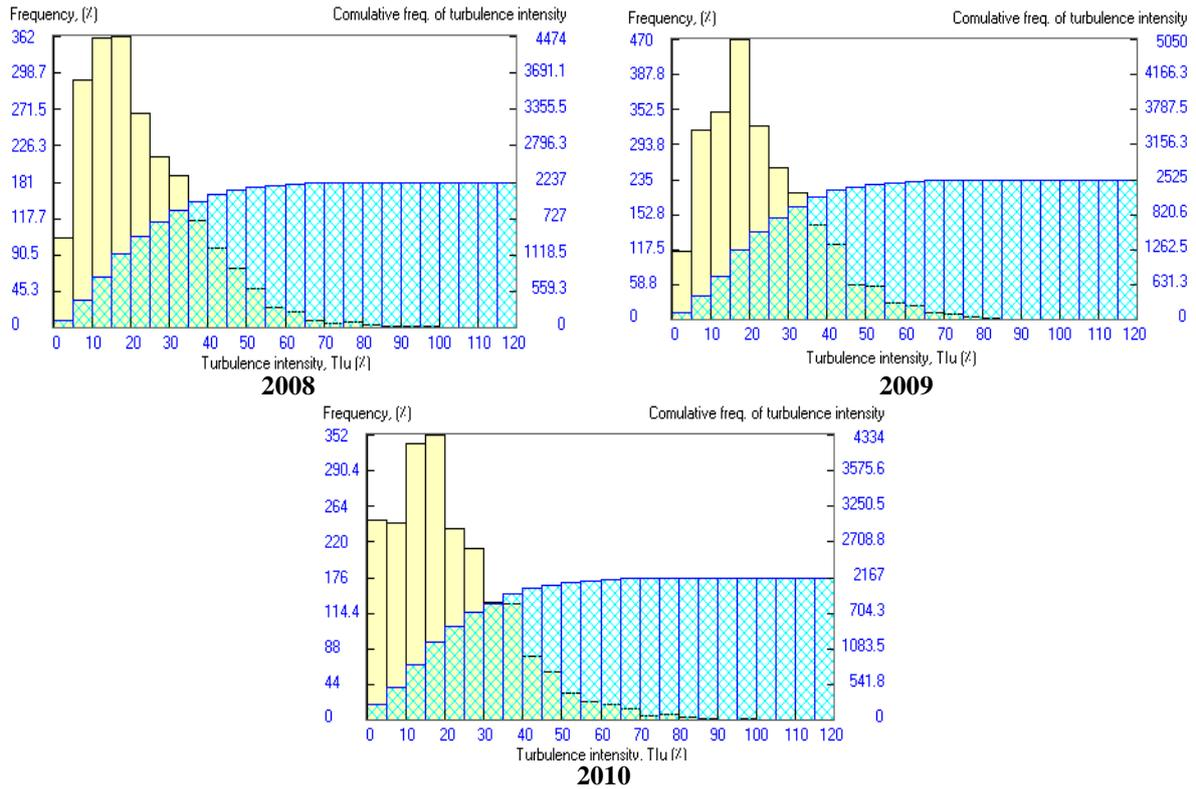
**Figure 7-** Frequency of turbulence intensity and its cumulative as a function of turbulence intensity belongs to Nasiriyah site for large and small wind turbine.
