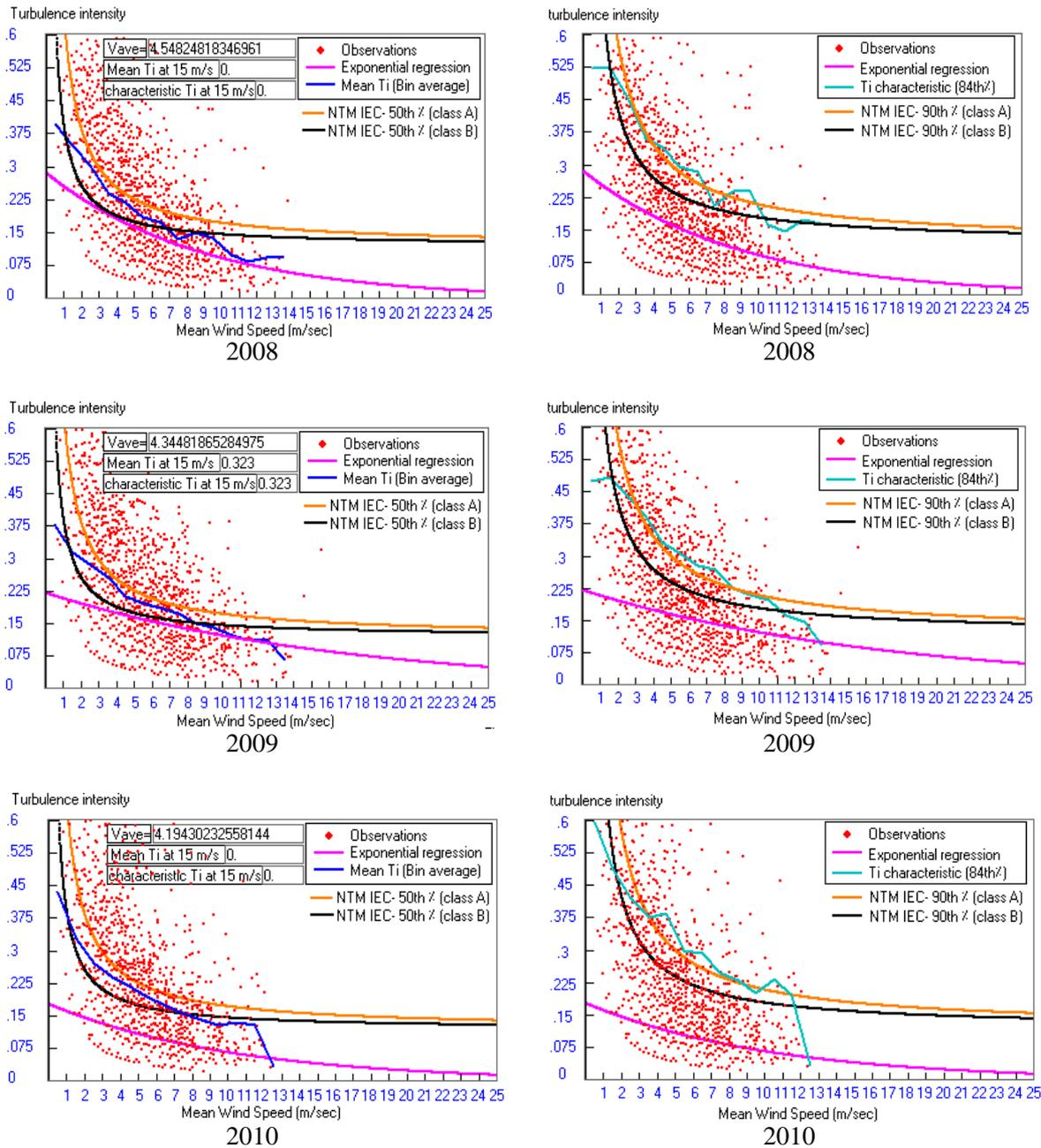
**Figure 6-** Turbulence intensity as a function of mean wind speed belongs to Nasiriyah site for small wind turbine.
