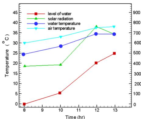
Figure. (11) The Temperature, solar radiation and the volume of distilled water distribution along the sunny day for 20/4/2016
