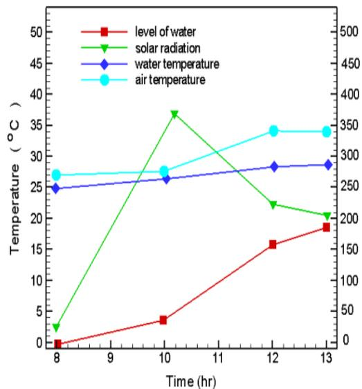
**Figure. (8) The temperature, solar radiation and the volume of distilled water distribution along the rainy and cloudy day for 10/4/2016.**
