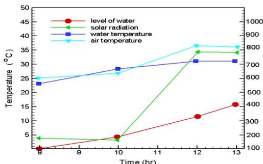
**Figure. (9) The Temperature, solar radiation and the volume of distilled water distribution along the rainy and partially cloudy day for 12/4/2016**
