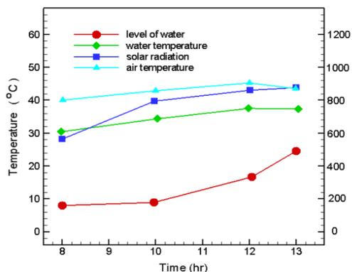
Figure. (12) The Temperature, solar radiation and the volume of distilled water distribution along the sunny day for 21/4/2016
