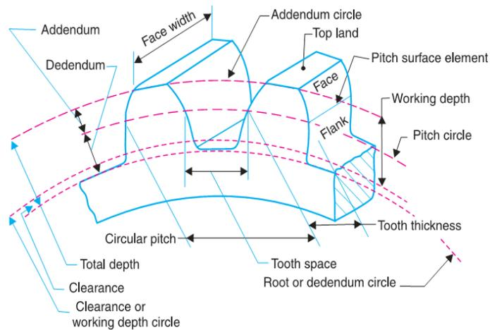
**Figure (2): Spur gear terminology [13].**
