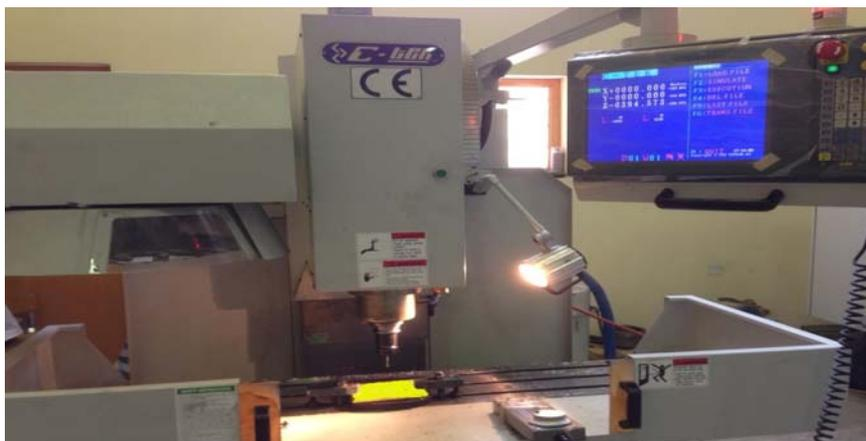
Figure (7) CNC milling machine
