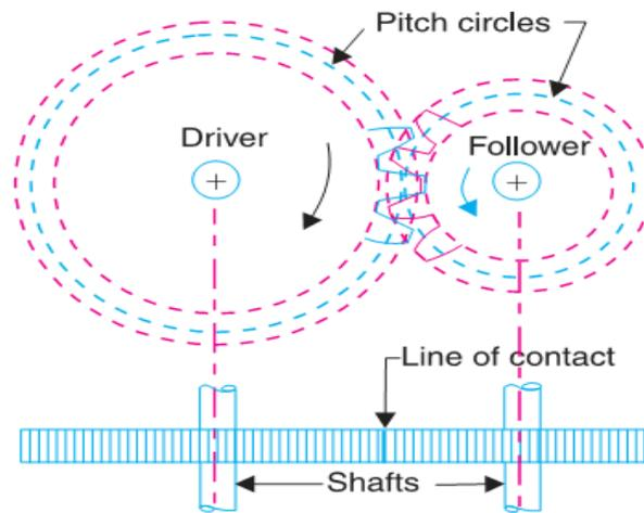
**Figure (1) Spur Gear [13]**
