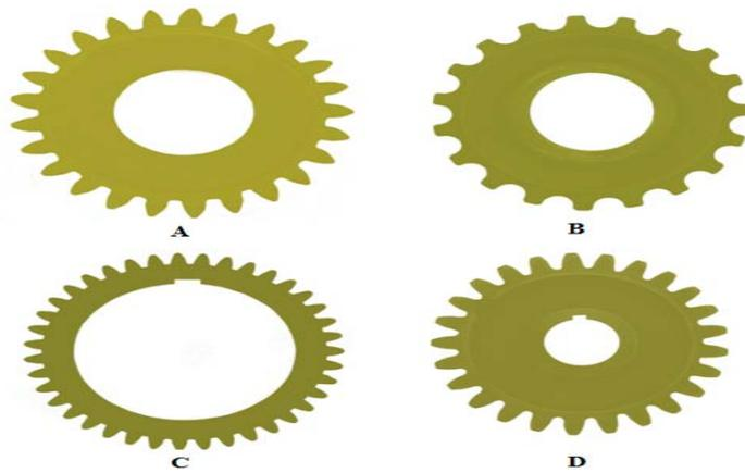
Figure (8) Spur Gears Manufactured
