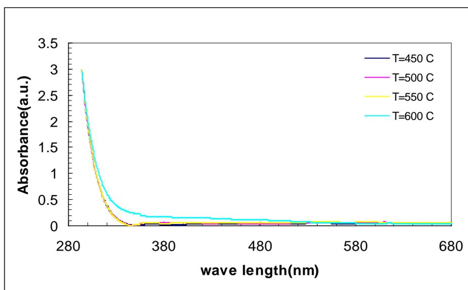
**Fig.(2):Absorption spectra of different annealing temperature (450,500,550, and 600 °C) of ZnS.**
