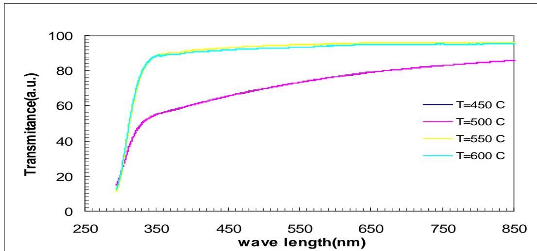
Fig. (4): Variation of transmittance (T) with wavelength ( $\lambda$ ) for ZnS at different temperatures (450, 500, 550 and 600°C) thin films.
