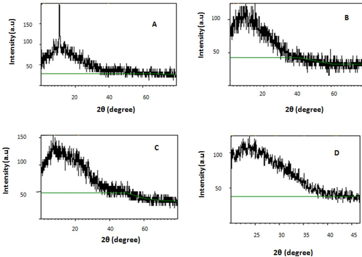
Fig.(1): x-ray at different annealing temperature(A- 450oC, B- 500°C, C-550°C, and D-600°C) between ( $2\theta$ ) and counts/sec
