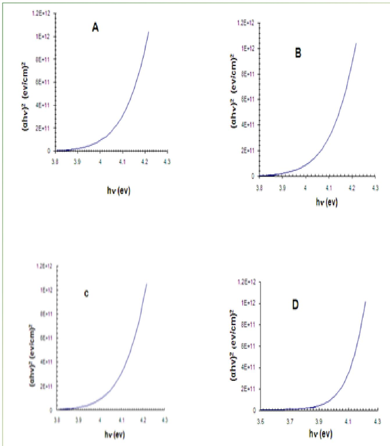
Fig. (3): Band gap determination of ZnS (A) T=450 °C, (B) T=500 °C, (C) T= 550 °C (D) T= 600 °C.
