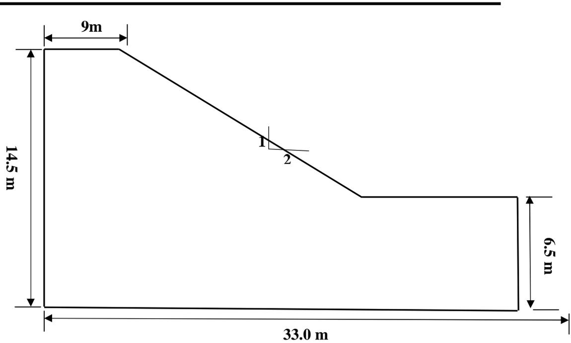
Figure (1): Cross section of road embankment.
