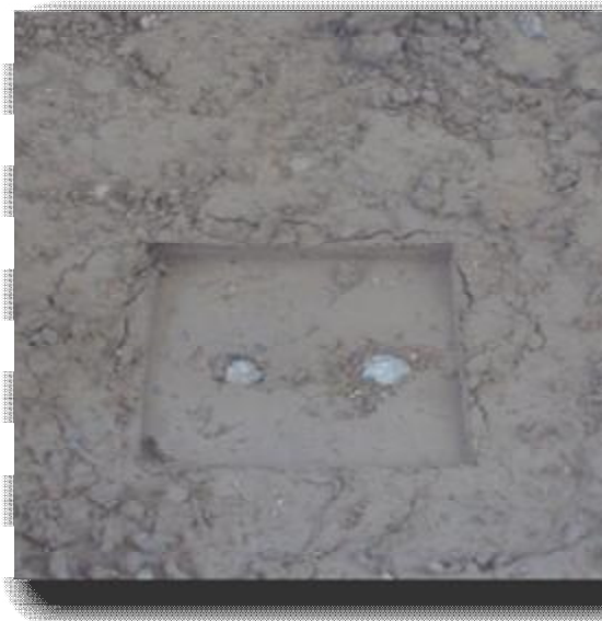
Plate (8) Two piles with raft after test.
