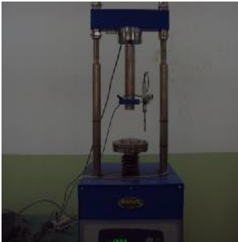
Plate (5) Load cell and indicator
