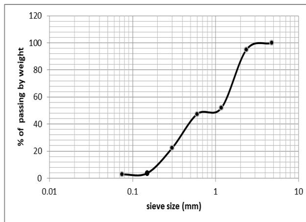
**Figure 4:** illustrates the grain size distribution of crushed bricks sand.
