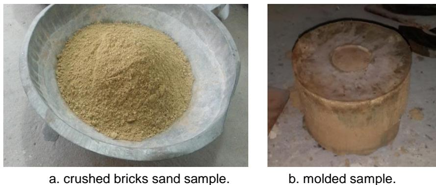
**Figure 2:** the crushed bricks sand material.
