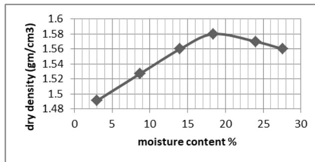
**Figure 5:** the moisture-density relationship of crushed bricks sand.
