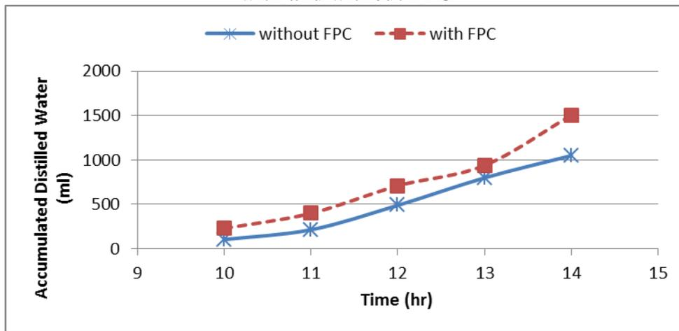
Fig. (9): Accumulative Fresh Water Productivity with and without FPC
