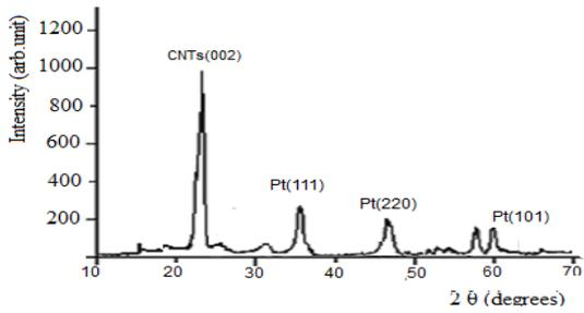
Figure 4. XRD analysis of (Pt :CNTs)
