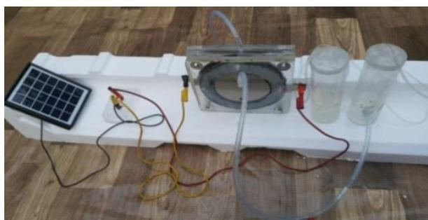
Figure 2. The electrolysis cell
