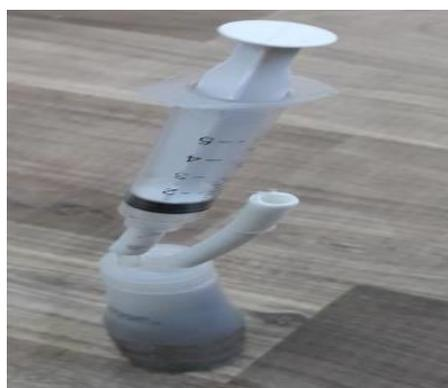
Figure 3. Hydrogen gas drying and storage system
