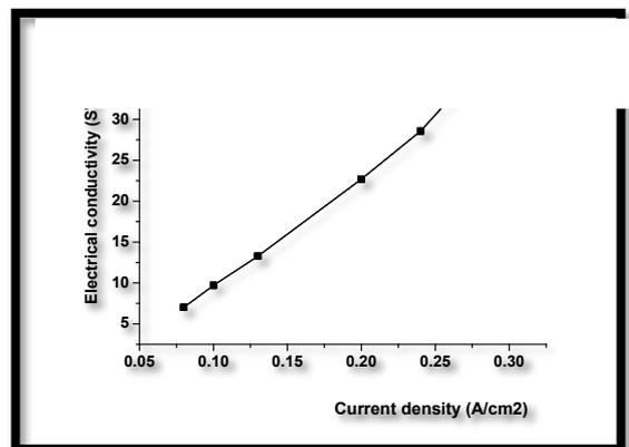
Figure 8. The relationship between current density -Electrical conductivity
