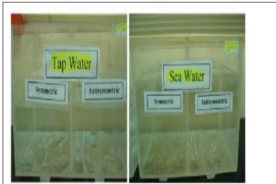
Figure (2) Seawater and tap water chambers
