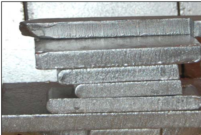
Fig. 6-A: shows improved samples of clean cut after removing HAZ only (no surface machining).
