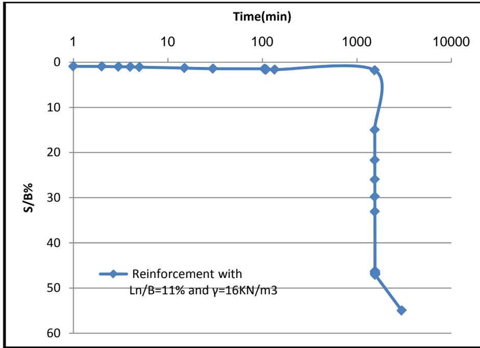
Fig (14) Time-S/B relation for reinforced model. 10% Saline soil applied stress=36.6KN/m<sup>3</sup>) Ln/B=11%,  $\gamma=16\text{KN/m}^3$  w.c=15%
