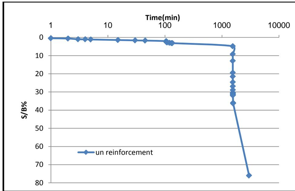
**Fig (7) Time-S/B relation for unreinforced model with 10% Saline soil, applied stress=36.6KN/m<sup>2</sup>,  $\gamma$ =14KN/m<sup>3</sup> w.c=15%**
