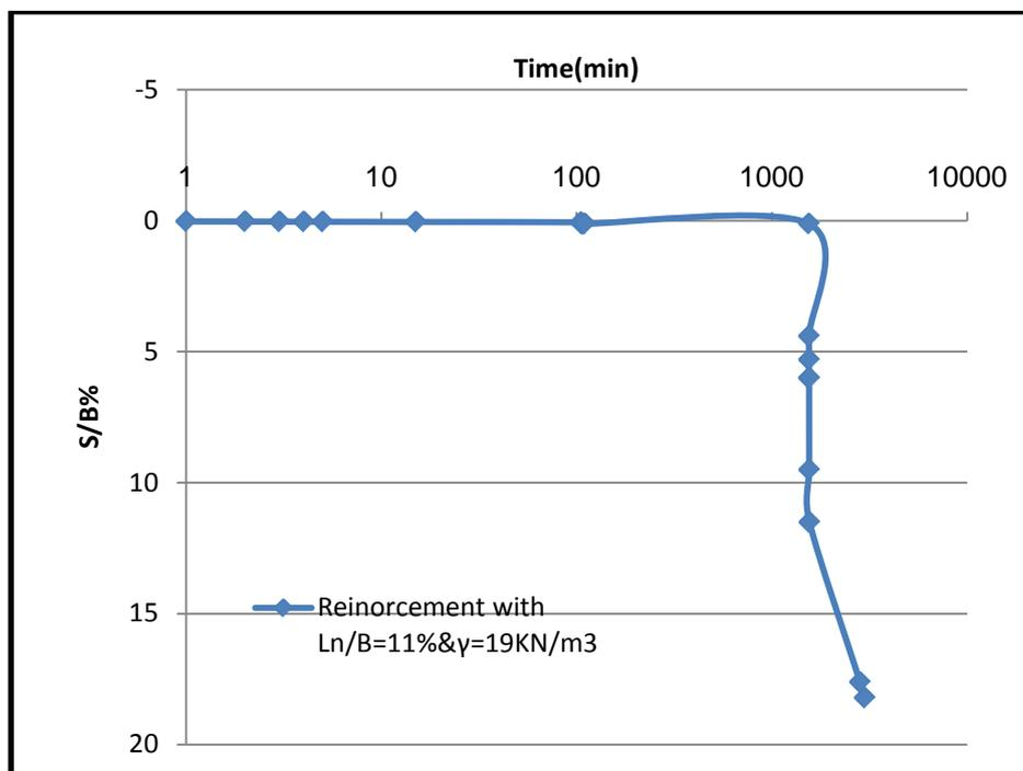
Fig (13) Time-S/B relation for reinforced model. With 10% Saline soil applied stress= $36.6\text{KN/m}^3$  &  $\gamma=19\text{KN/m}^3$
