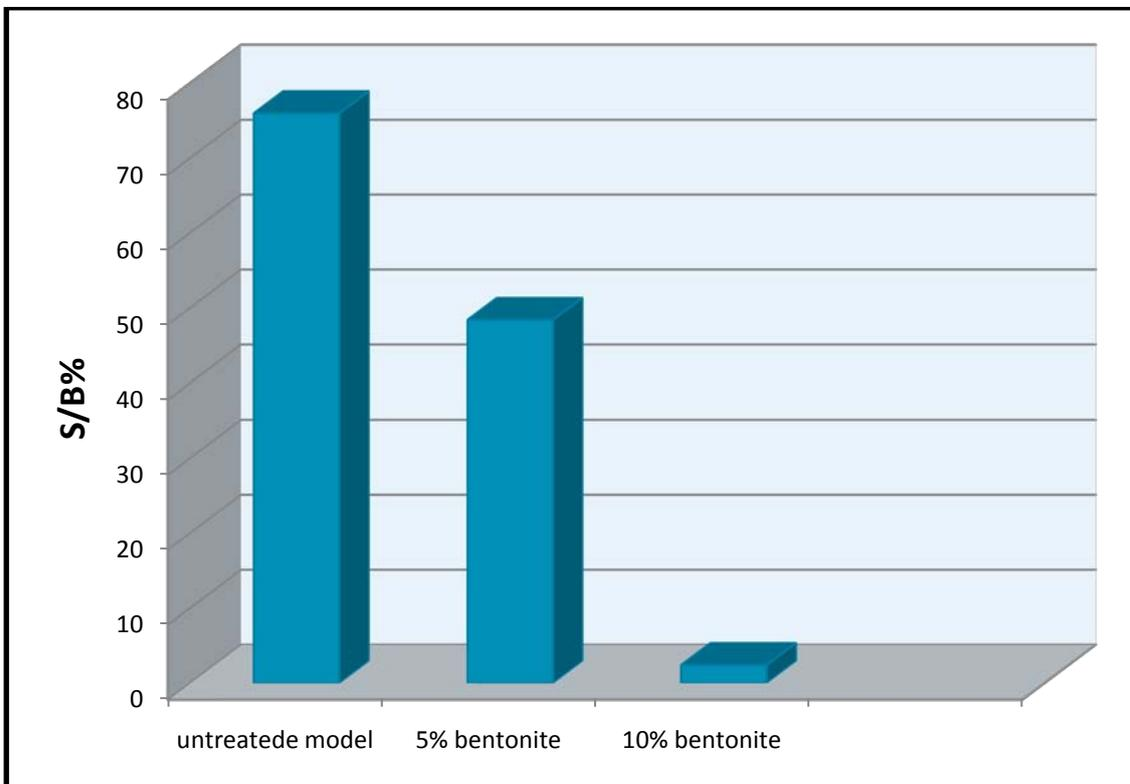
Fig (24) monograph shows the improvement of saline soil by bentonite ( $\gamma$ =14KN/m<sup>3</sup>, 10% Salinity and vertical stress=36.6KN/m<sup>2</sup>).
