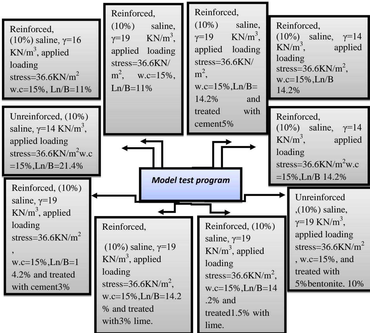
**Fig(1): Testing program flowchart**
