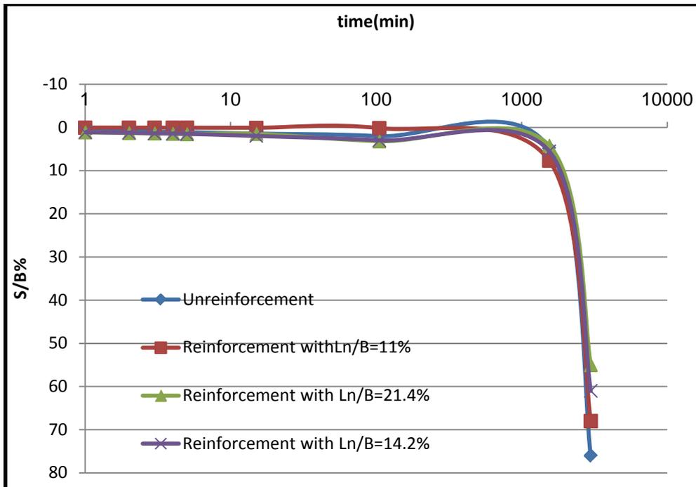
Fig (12) Treatment of saline soil by physical treatment (Ln/B=11%, 14.2% and 21.4%),  $\gamma=14\text{KN/m}^3$ , w.c=15% and stress= $36.6\text{KN/m}^3$
