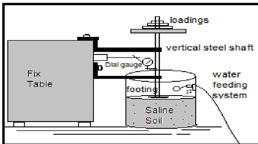
Fig(4): diagram of loading frame and model preparation steps
