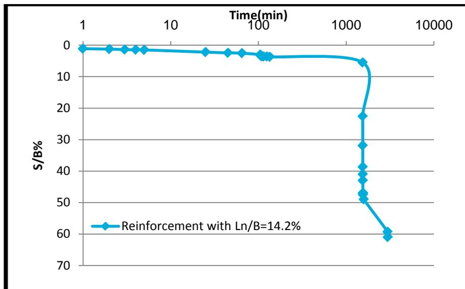
Fig (9) Time-S/B relation for reinforced model. With 10% Saline soil applied stress= $36.6\text{KN/m}^3$ ),  $\gamma=14\text{KN/m}^3$   $L_n/B=14.2\%$  and w.c=15%
