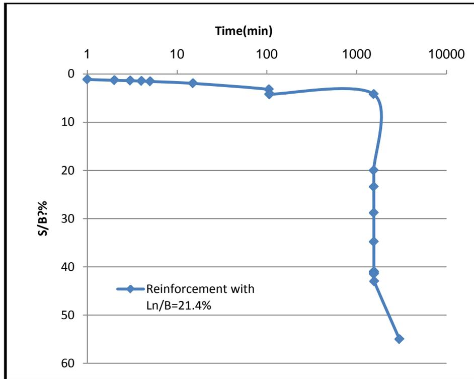
**Fig (10) Time-S/B relation for reinforced model. With 10% Saline soil applied stress=36.6KN/m<sup>3</sup>) Ln/B=21.4%,  $\gamma$ =14KN/m<sup>3</sup>, w.c=15%**
