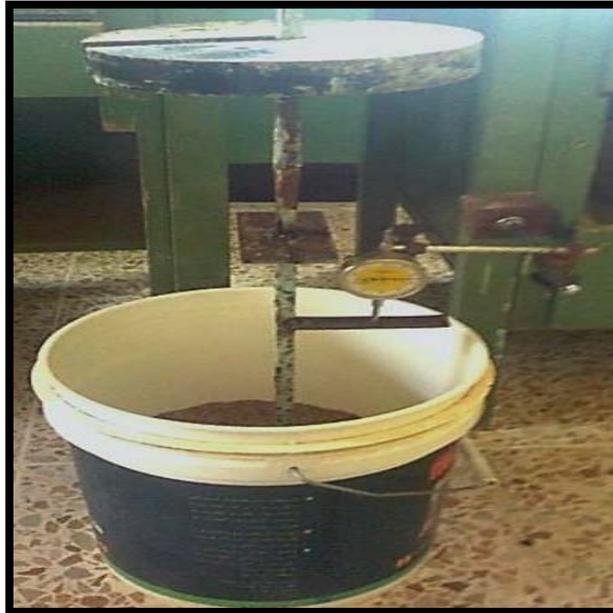
**Fig (5) : A picture for the manufactured laboratory model and the fix loading system, used in the study.**
