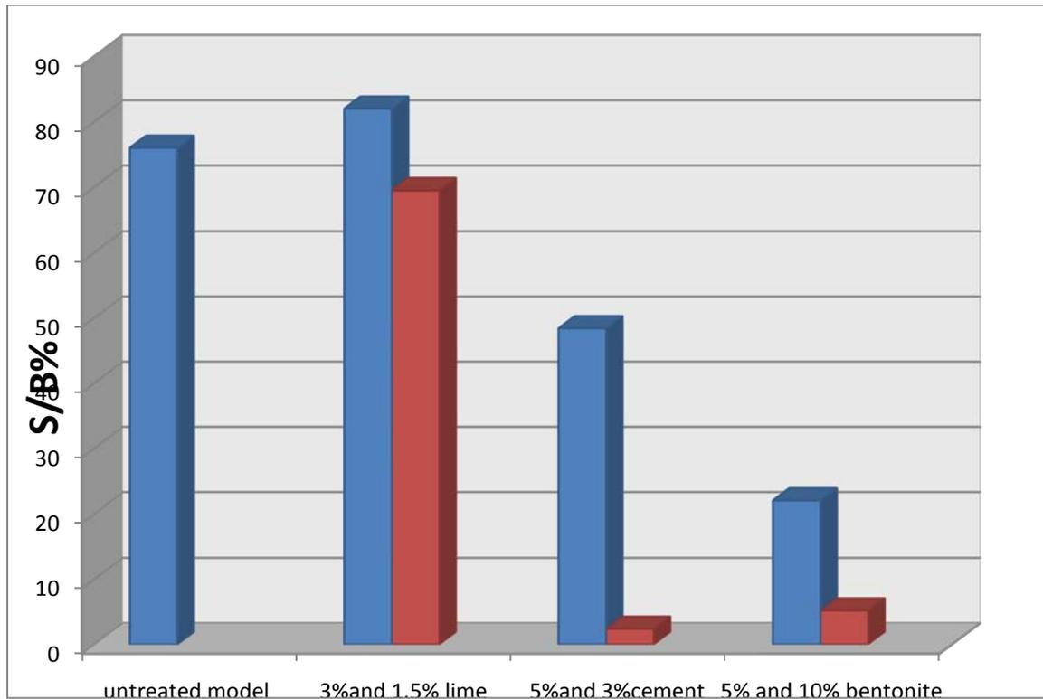
**Fig (22): Effect of chemical additives with reinforced on collapsibility of saline soil ( $\gamma=14\text{KN/m}^3$ , 10% salinity and stress effect= $36.6\text{KN/m}^2$ )**
