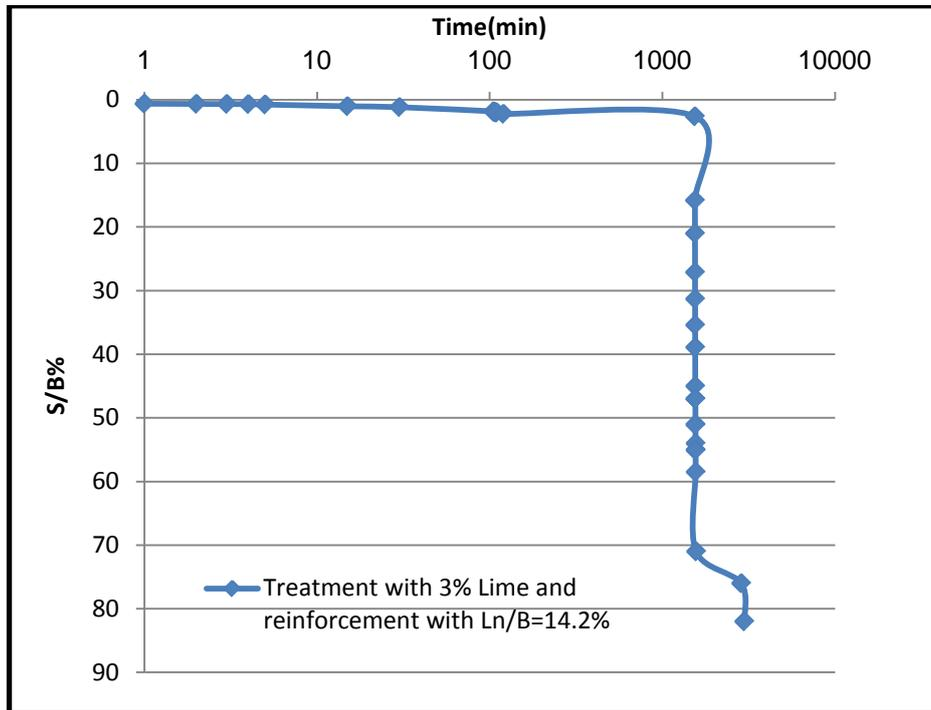
Fig (18) time-S/B relation for reinforced model. With 10% Saline soil, applied stress=36.6KN/m<sup>3</sup> Ln/B=14.2%,  $\gamma=14$ KN/m<sup>3</sup> (lime3%) and w.c=15%
