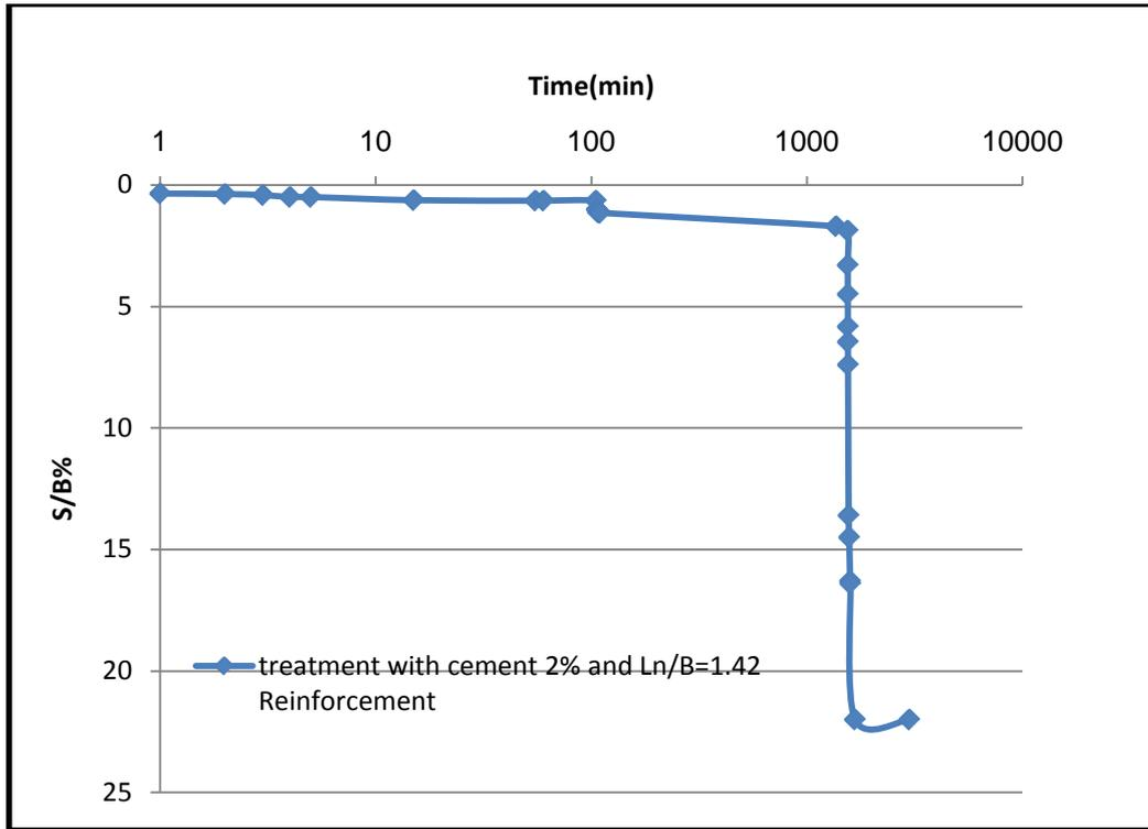
Fig (19) Time-S/B relation for reinforced model. Saline soil 10%, applied stress=36.6KN/m<sup>3</sup> Ln/B=14.2%,  $\gamma$ =14KN/m<sup>3</sup> (cement2%) and w.c=15%
