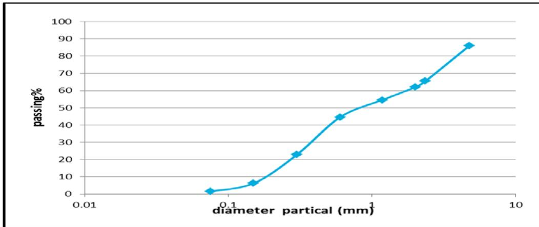
**Fig (2) grain size distribution curve for soil used.**
