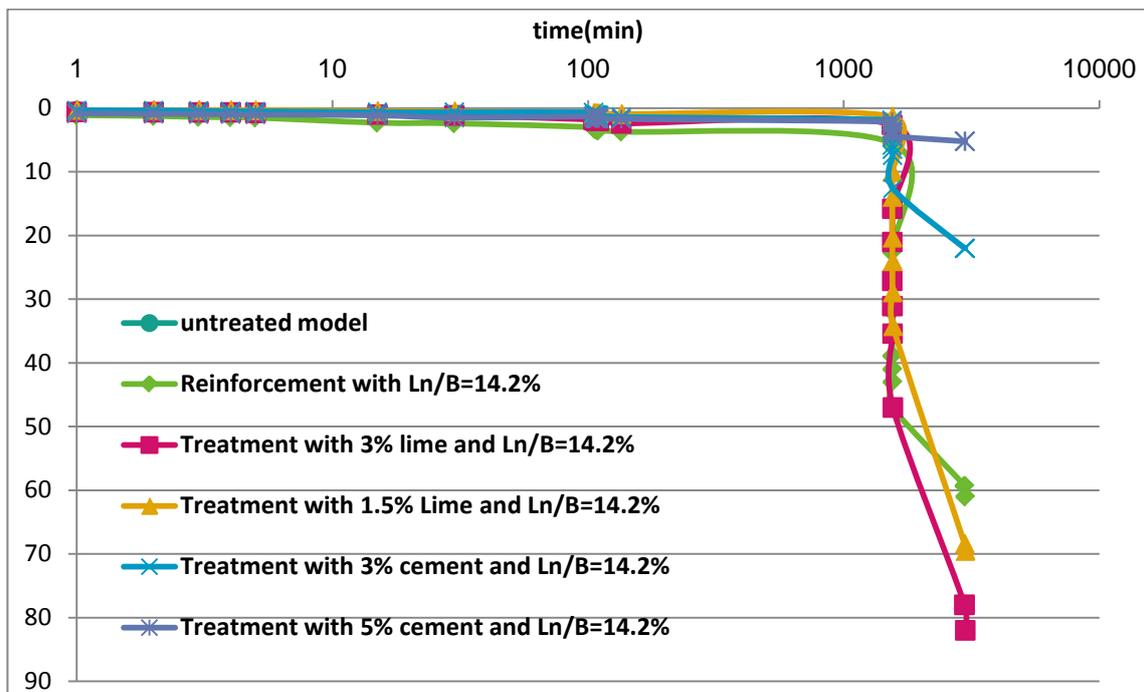
Fig (21) Treatment saline soil by chemical and physical treatment, ( $\gamma=14\text{KN/m}^3$ ,  $w.c=15\%$  and  $Ln/B=14.2\%$ )
