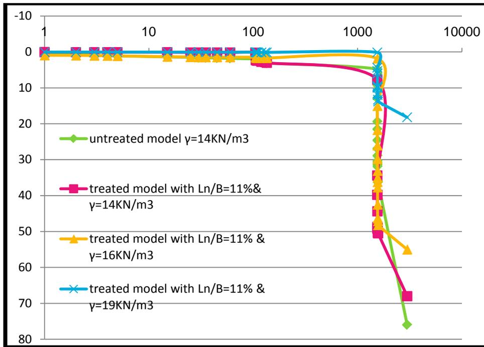
Fig (15) Treatment of saline soil with different density by physical treatment (Ln/B=11%) , compacted with different soil densities 14, 16 and 19 kN/m<sup>3</sup>.
