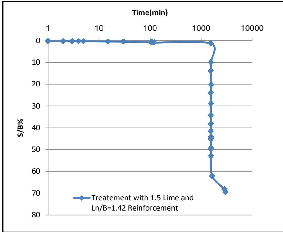
Fig (17) Time-S/B relation for reinforced model. Saline soil 10%, applied stress=36.6KN/m<sup>3</sup> Ln/B=14.2%,  $\gamma=14$ KN/ (lime 15%) and w.c= 15%
