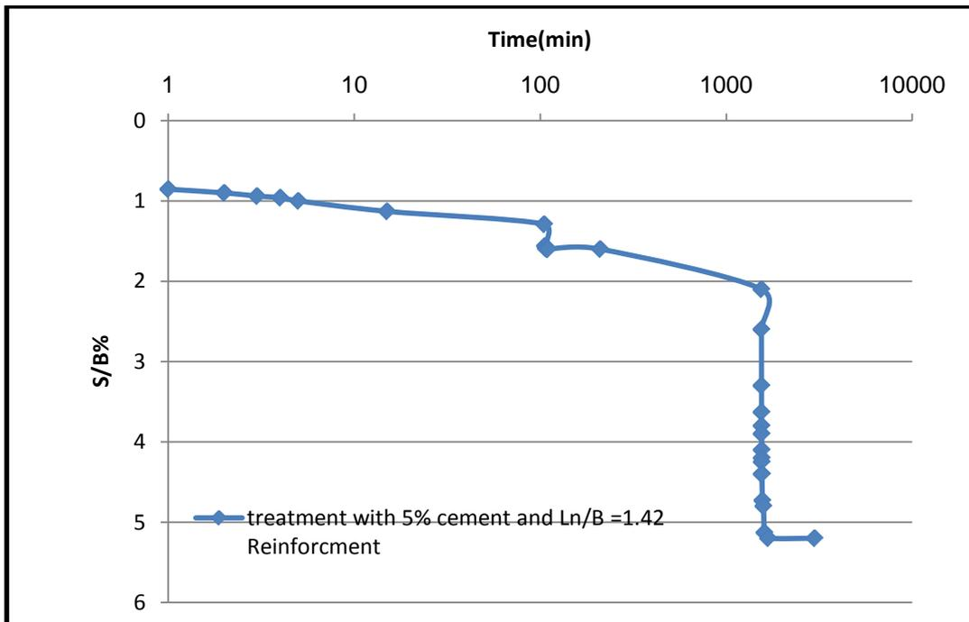
Fig (20) Time-S/B relation for reinforced model.10% Saline soil applied stress=36.6KN/m<sup>3</sup> Ln/B=14.2%,  $\gamma$ =14KN/m<sup>3</sup> (cement5%) and w.c=15%
