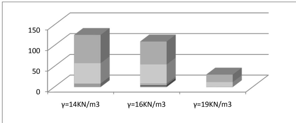
**Fig (16): Monograph of the effect of compaction of saline soil and reinforcement with ( $L_n/B=11\%$ )**
