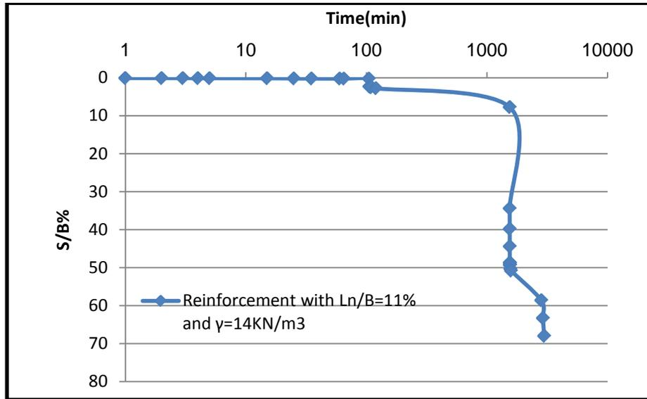
Fig (8) Time-S/B relation for reinforced model. With 10% Saline soil applied stress= $36.6\text{KN/m}^3$ )  $L_n/B=11\%$ ,  $\gamma=14\text{KN/m}^3$ , w.c=15%
