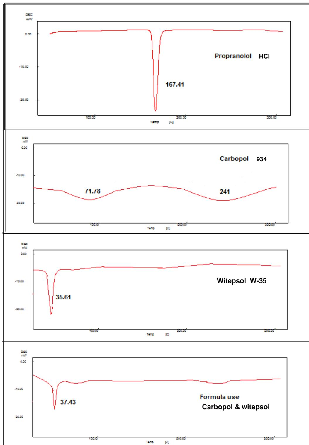
Figure (5) DSC thermograms of propranolol HCl, carbopol 934, witepsol W-35 and formula contains carbopol and witepsol
