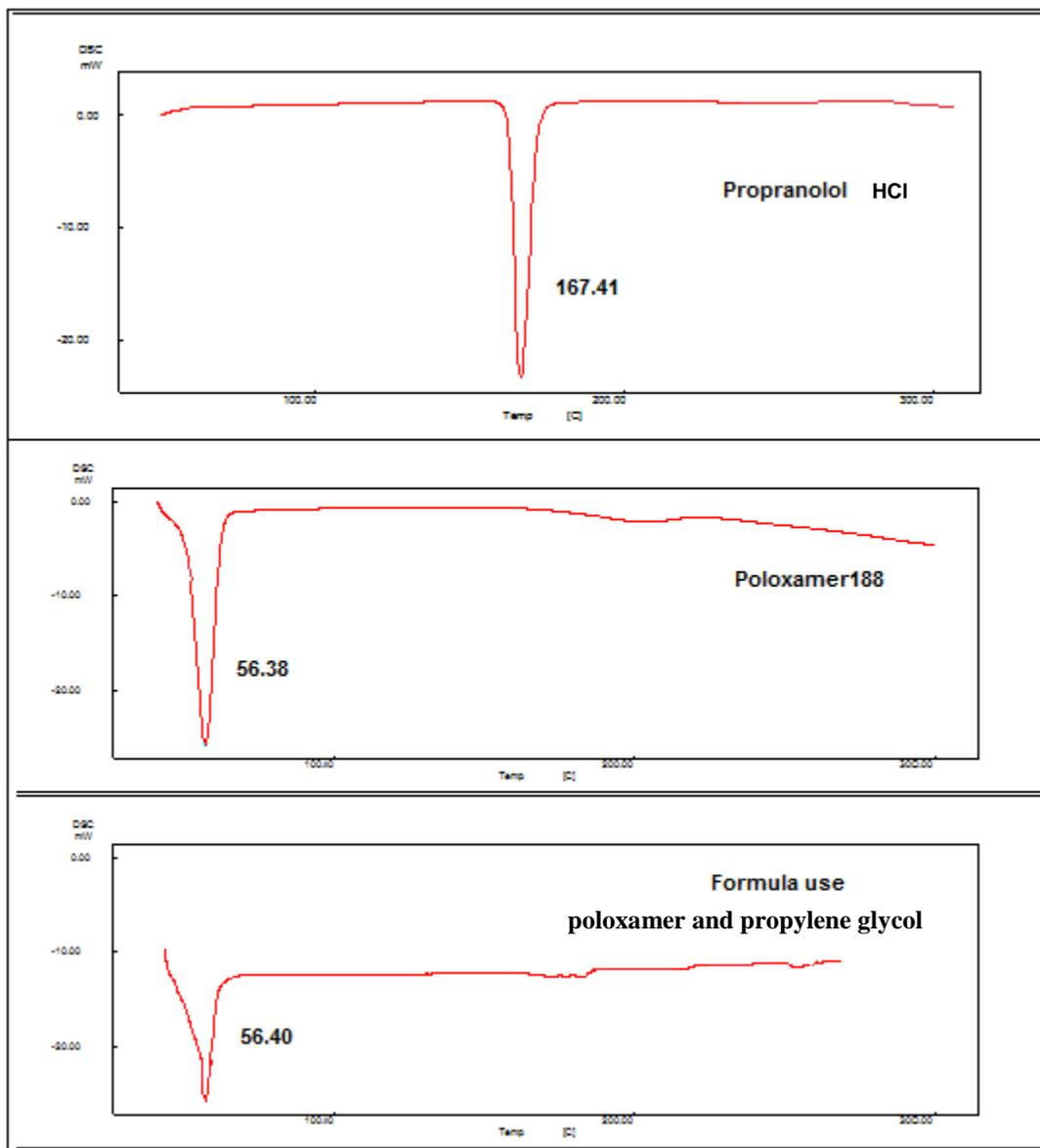
Figure (7) DSC thermograms of propranolol HCl, poloxamer188, and formula contains poloxamer and propylene glycol
