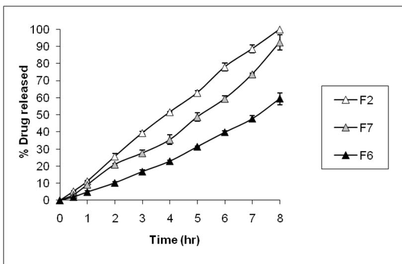
Figure (3):- Effect of addition of carbopol 934 to PEG 4000 based suppositories on the dissolution of propranolol HCl in pH 6.8 at  $37 \pm 0.5^\circ\text{C}$
