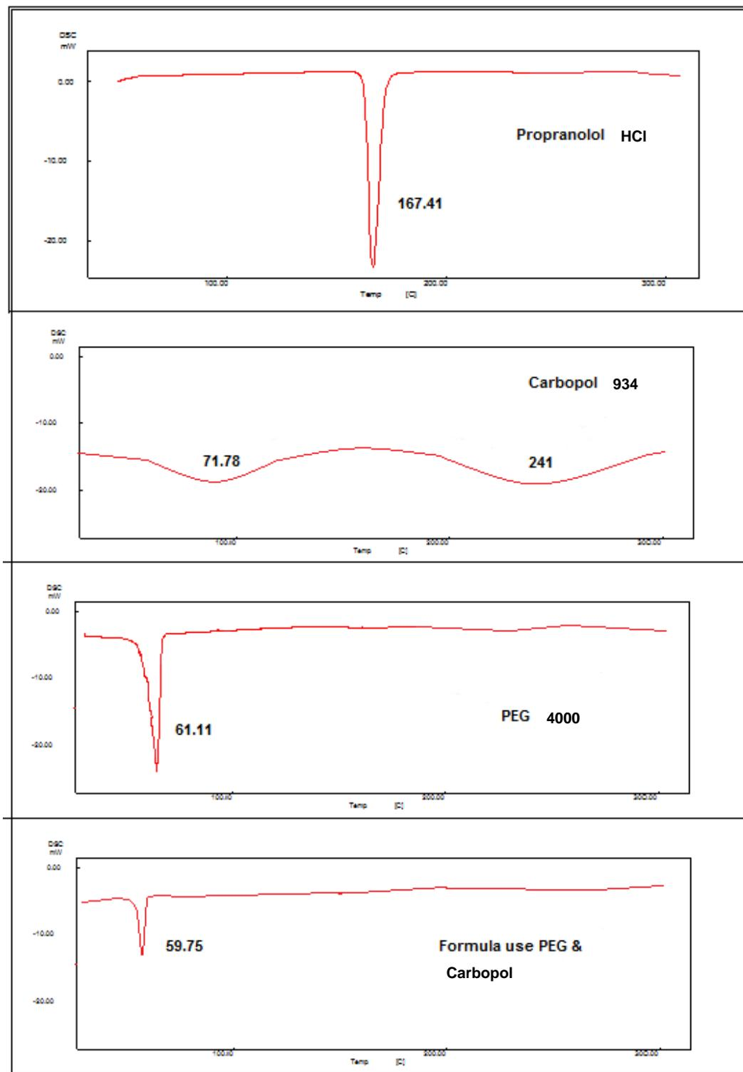
Figure(6) DSC thermograms of propranolol HCl, carbopol 934, PEG 4000 and formula contains PEG and carbopol
