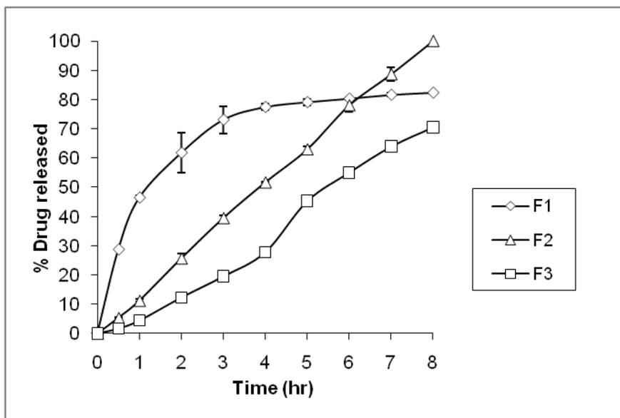
Figure (1):-Effect of type suppository base on the dissolution of propranolol HCl in pH 6.8 at 37±0.5°C
