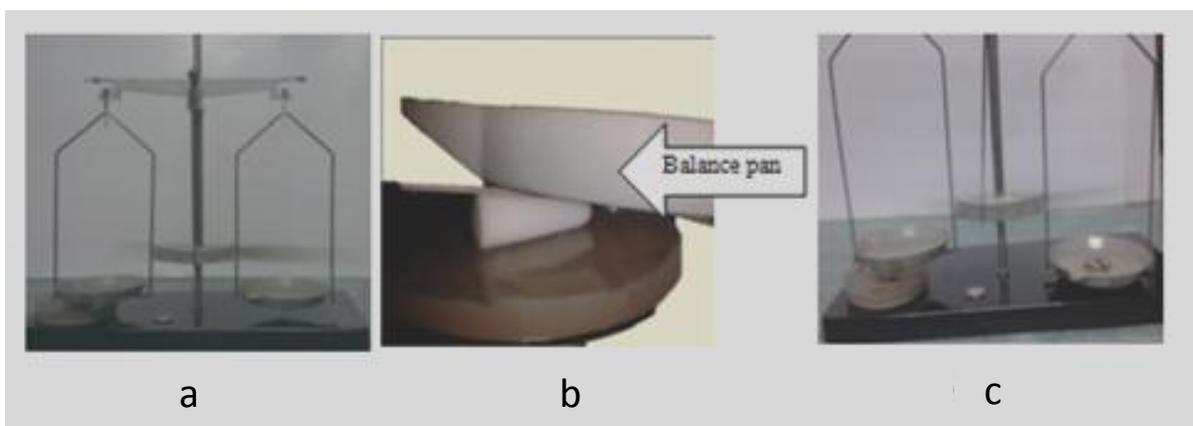
Photo (1):- Photography of simple modified balance for mucoadhesion strength study (a,b. attached suppository, c. detached suppository)
