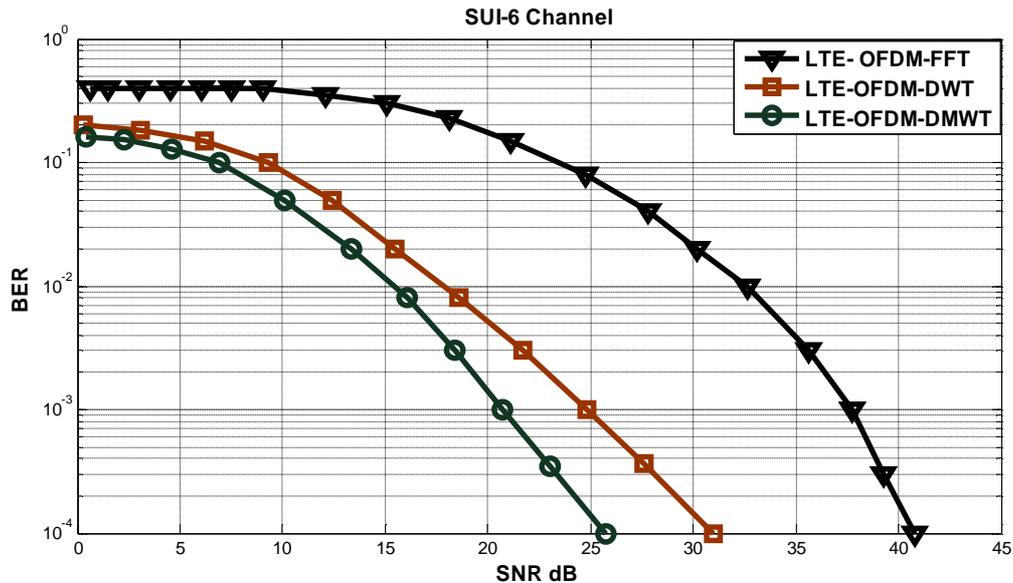
**Fig .(7) BER performance of LTE Transceiver based OFDM DMWT in SUI-6 Channel**
