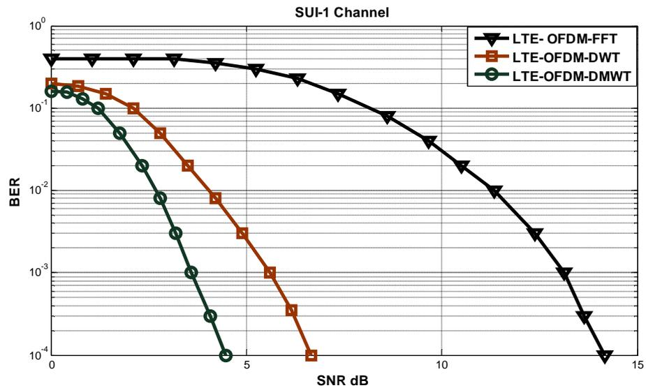
Fig .(2) BER performance of LTE Transceiver based OFDM DMWT in SUI-1 Channel
