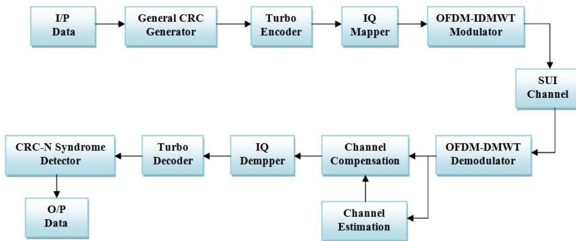
Fig .(1) Block Diagram of Proposed Modified LTE Transceiver Structure
