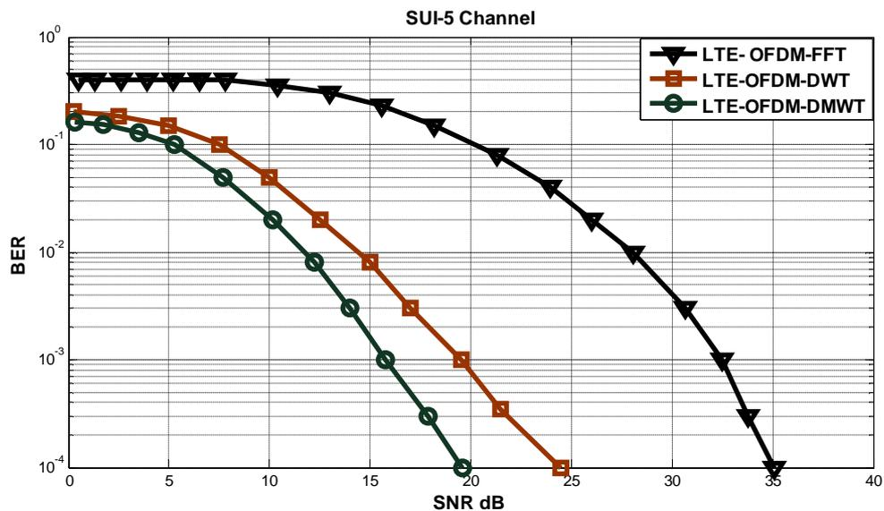
Fig .(6) BER performance of LTE Transceiver based OFDM DMWT in SUI-5 Channel
