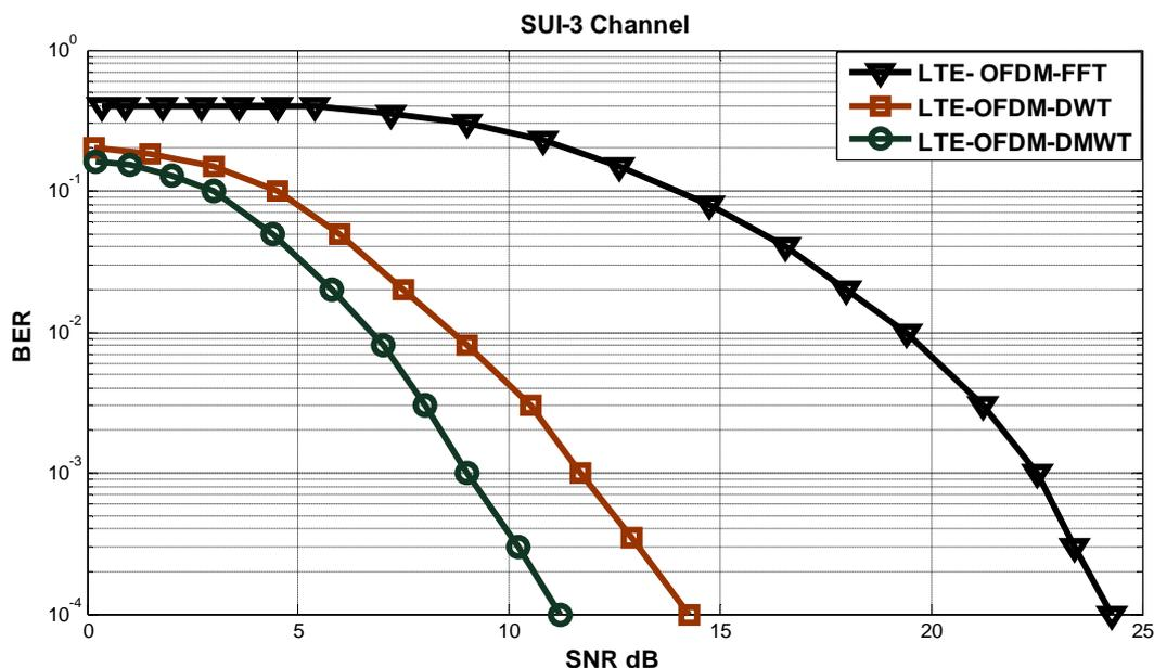
Fig .(4) BER performance of LTE Transceiver based OFDM DMWT in SUI-3 Channel
