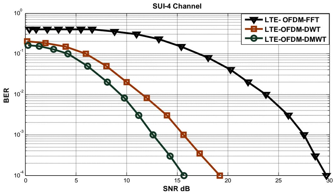
Fig .(5) BER performance of LTE Transceiver based OFDM DMWT in SUI-4 Channel
