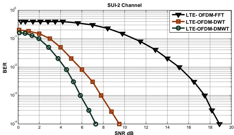
Fig .(3) BER performance of LTE Transceiver based OFDM DMWT in SUI-2 Channel
