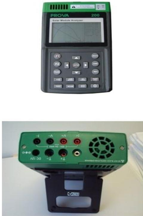
Fig.3 :The Prova 200 solar panel analyzer
