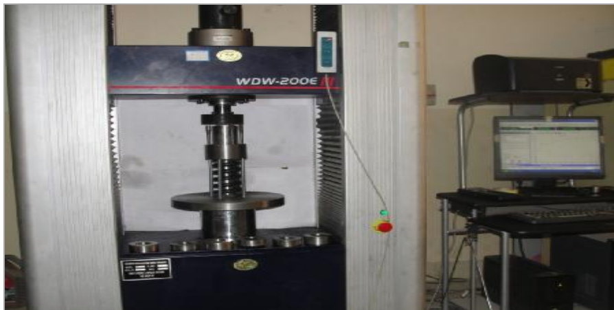
Figure (4) Deep drawing die attached to computerized testing machine.
