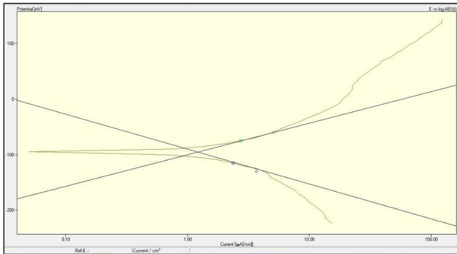
Figure 4: Polarization curve of mild steel in acid solution at 25°C containing 300 ppm of green inhibitor
