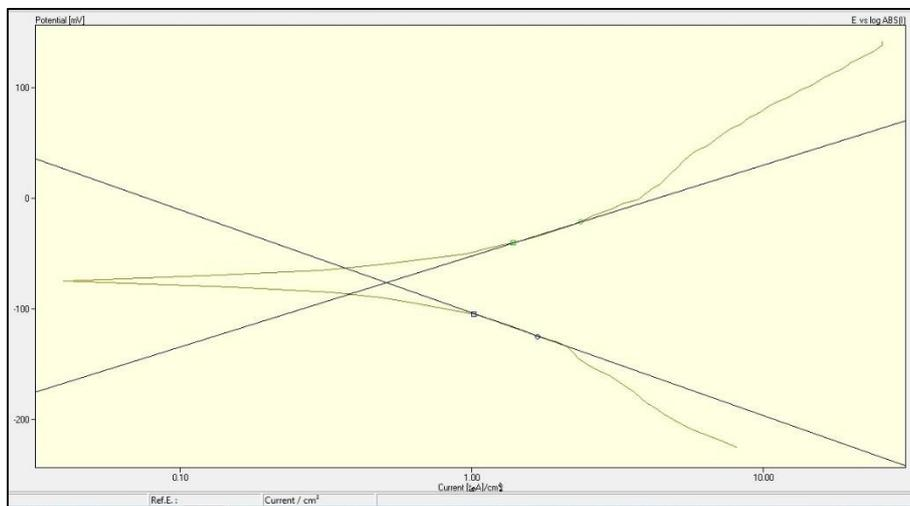
Figure 11: Polarization curve of mild steel in acid solution at 25°C containing 1000 ppm of green inhibitor
