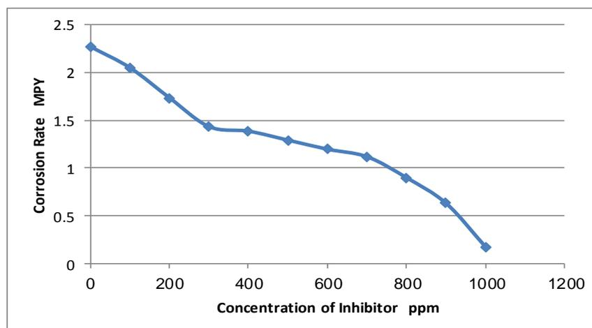
**Figure 12: corrosion rate of of mild steel in 1 M H<sub>2</sub>SO<sub>4</sub> with different concentration of green inhibitor at room temperature**
