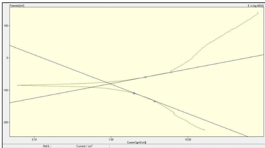
Figure 5: Polarization curve of mild steel in acid solution at 25°C containing 400 ppm of green inhibitor
