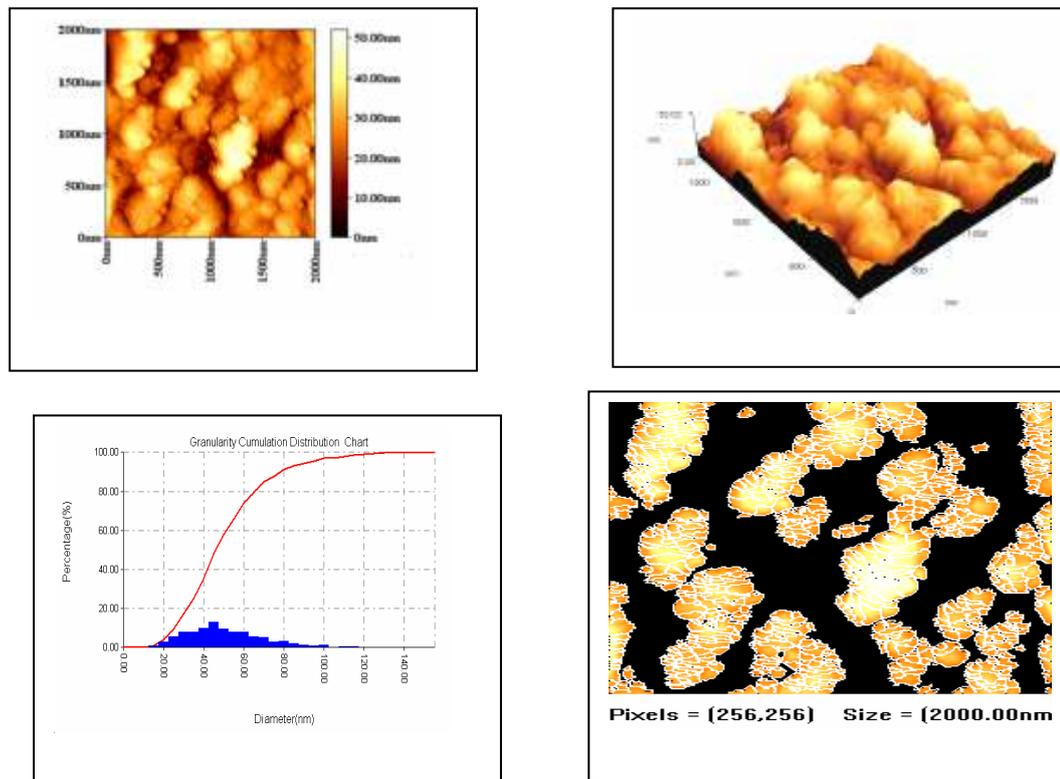
**Figure (8) Represents the AFM micrograph of  $\text{In}_2\text{O}_3$  films deposited at the highest energy of (400 mj).**
