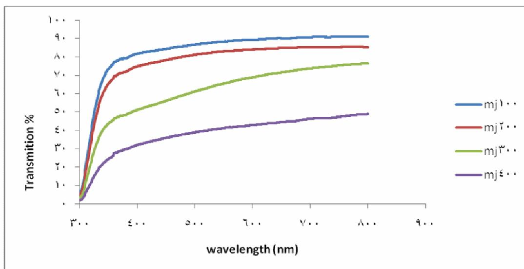
**Figure (3) Optical transmission as a function of wavelength for  $\text{In}_2\text{O}_3$  at different laser power density between(100-400) mj /pulse.**
