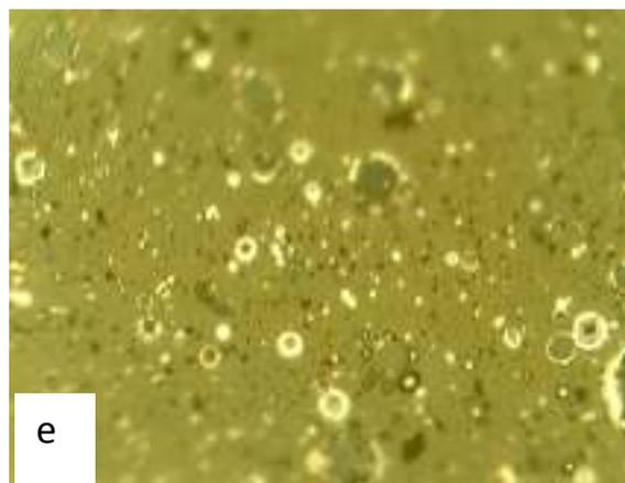
**Figure (2) Surface morphology of  $\text{In}_2\text{O}_3$  samples prepared at room temperature and different laser energies (a- 100mj b- 200mj c- 300mj d- 400mj e- 500mj) and laser fluence of ( $89.17\text{J}/\text{cm}^2$ ),  $\times=1000$  for all pictures.**
