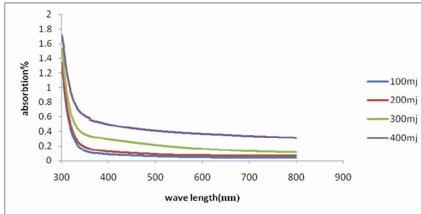
**Figure (4) Optical absorption as a function of wavelength for  $\text{In}_2\text{O}_3$  at different laser power density between(100-400) mj /pulse**
