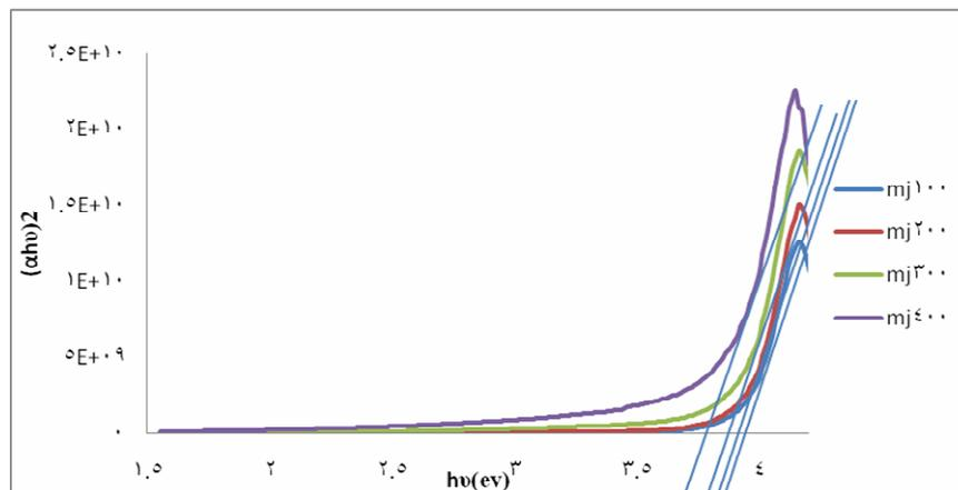
**Figure(5)  $(\alpha h\nu)^2$  (eV/ cm)<sup>2</sup> vs.  $h\nu$ (ev) of  $\text{In}_2\text{O}_3$  NPs at different laser power density.**
