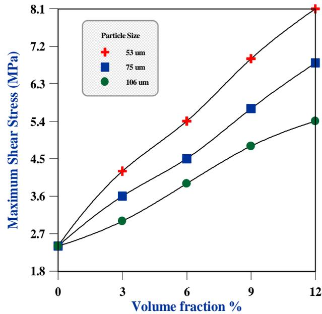
Figure (8): shown the effect of volume fraction on maximum shear stress
