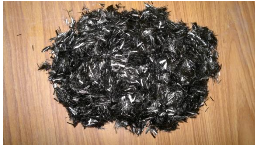
Plate (2) Discrete carbon fibers used in the present study.
