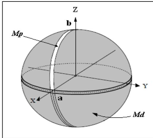
Figure 7 Net effects of the four mating faces. (Mp) portion shows DOFs [the arc (ab) only]
