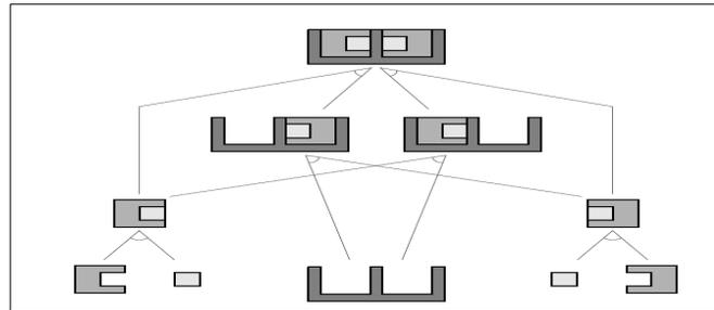
Figure 1 Example of an AND/OR disassembly graph [Romney, 1997].
