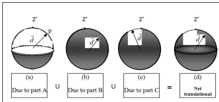
Figure 15 Translation constraints for the parts
