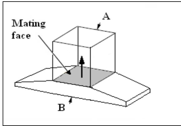
Figure 4 An object with single mating face
