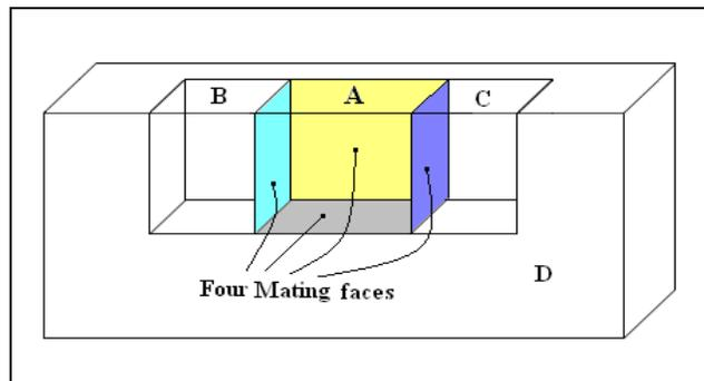
Figure 6 Object A has four mating faces
