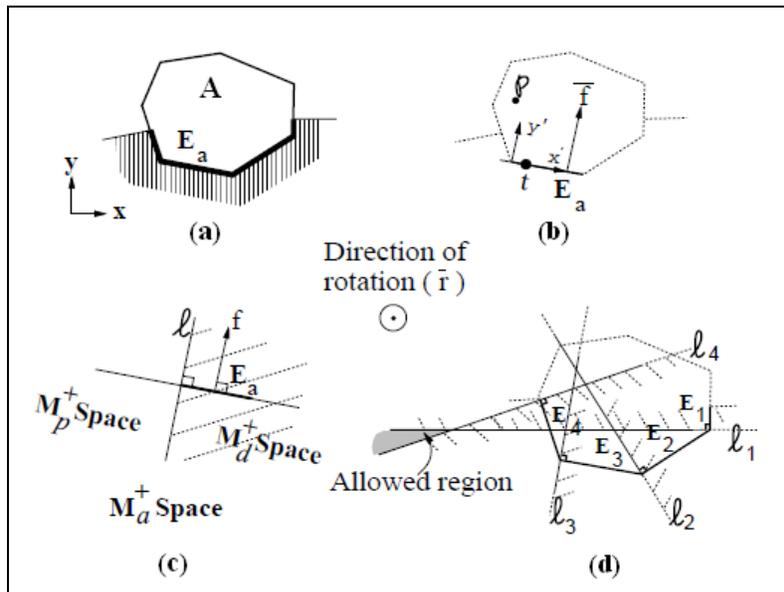
Figure 8 Rotational restraints on planar objects (a) A polygon with its mating conditions, (b) A single mating element  $E_a$ , (c) Anticlockwise rotation is disallowed about axes that lie in the shaded region, (d) Superposition of individual constraints due to contact over edges [Mattikalli & Khosla, 1992]
