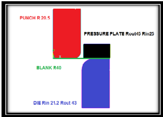
Figure (1) Finite element model of the sheet material and drawing (A) cylindrical die and punch (B) Hexagonal die and punch
