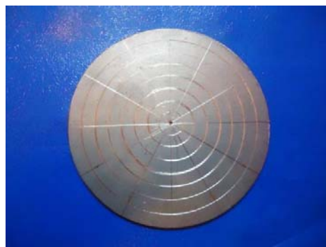
Figure (4) The blank with grids, by using mechanical grid marker
