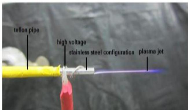
Figure (1) Photograph at working of the non-thermal atmospheric pressure plasma torch
