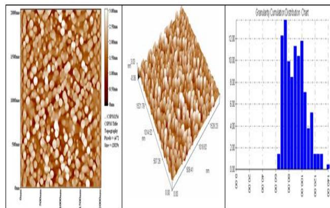
Figure (10) AFM photographs of PMMA/ZnS thin film at 7wt.% ZnS: 2D image, 3D image and granularity accumulation distribution chart
