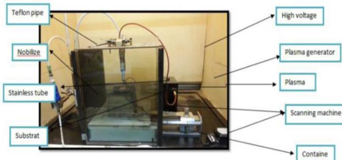
Figure (2) Photograph for the non-equilibrium atmospheric pressure plasma system for PMMA/ZnS nanocomposite thin films preparations
