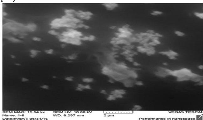
Figure (9) SEM image for PMMA/ZnS nanocomposite film at 7wt.% ZnS NPs concentration
