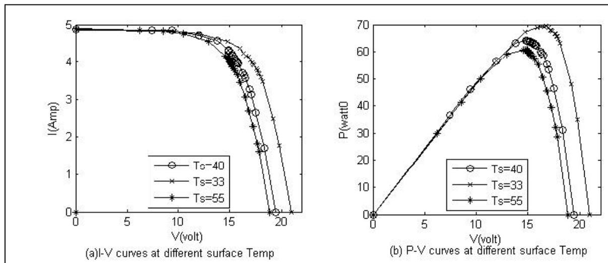
Fig. (1) a I-V curves at different surface temperature.
