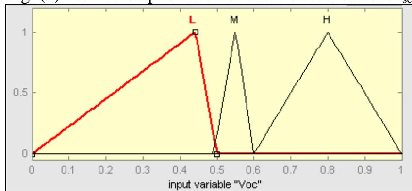
Fig. (5) Membership function of open circuit voltage  $V_{oc}$ .
