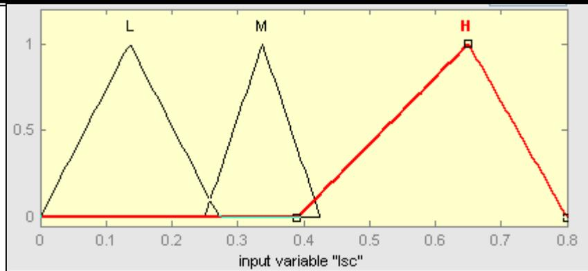
Fig. (4) Membership function of short-circuit current  $I_{sc}$ .
