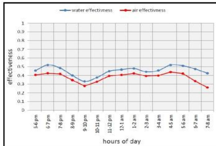
Figure (10) air and water heat exchanger effectiveness
