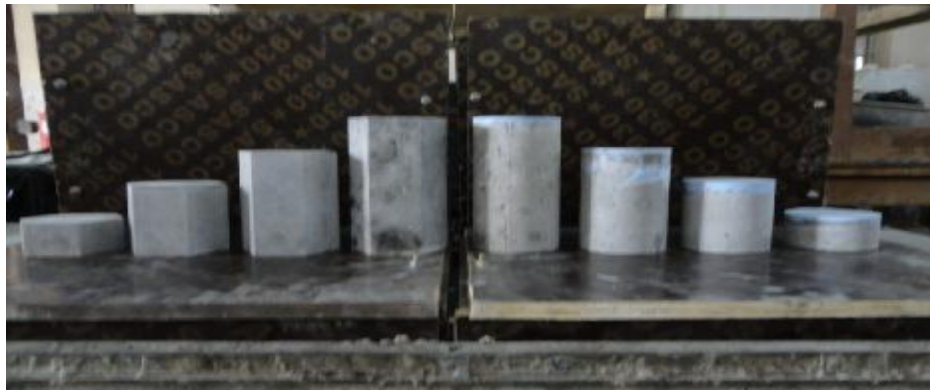
Plate 3: Hexagonal and cylindrical specimens of various sizes
