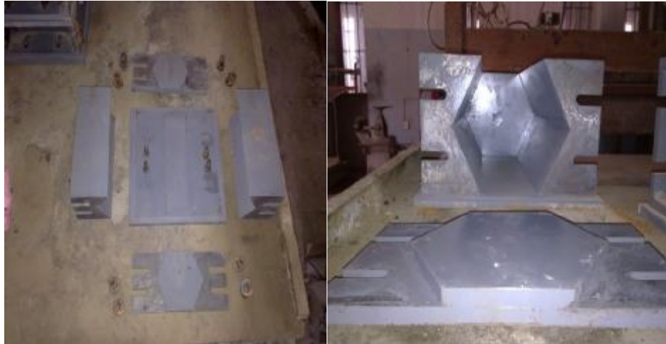
Plate 1: Mould assembly of the hexagonal specimens
