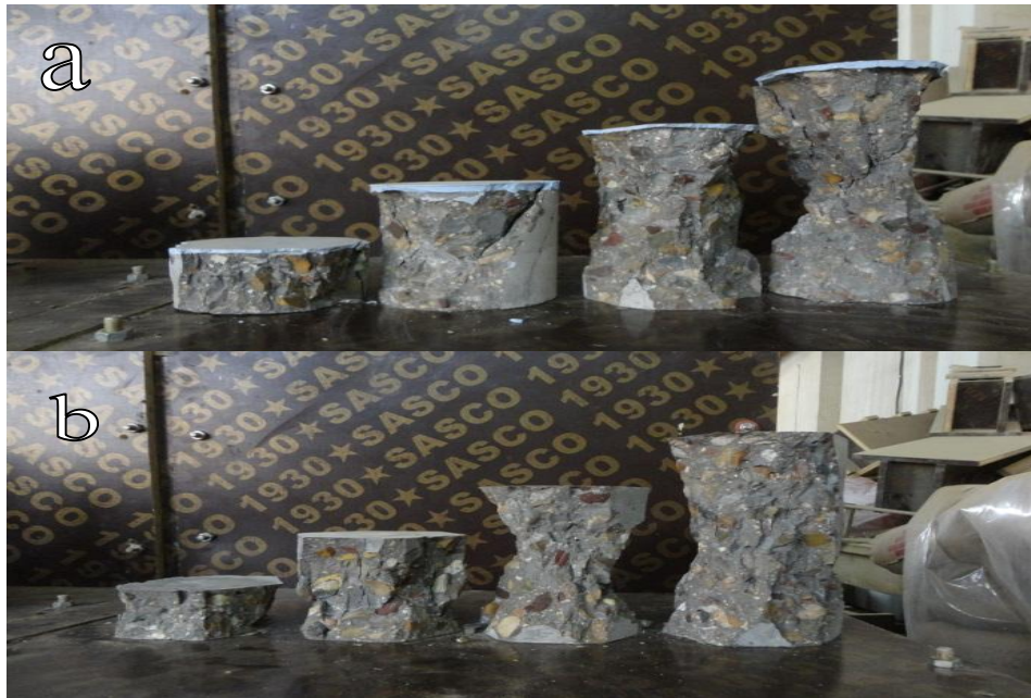
Plate 4: Fracture failure for a) cylindrical specimens and b) hexagonal specimens with different H/D ratios; where H/D being 2, 1.5, 1, and 0.5.
